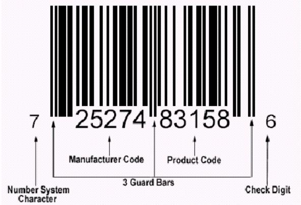
Another importation detail of barcodes is the Number Character System which is used to specify how the barcode is being used and as we will see later with EAN barcodes how they determine the way the numbers are encoded. Here is a breift list of Codes of the Number System Character:
