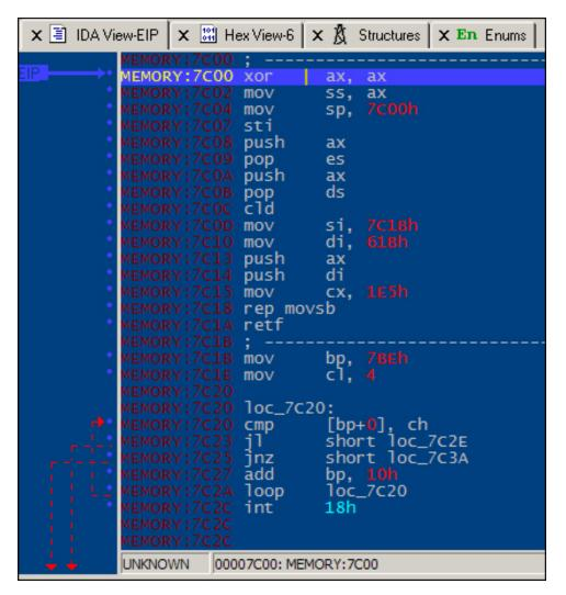
Figure 4. Debugging of boot code in IDA Pro.
