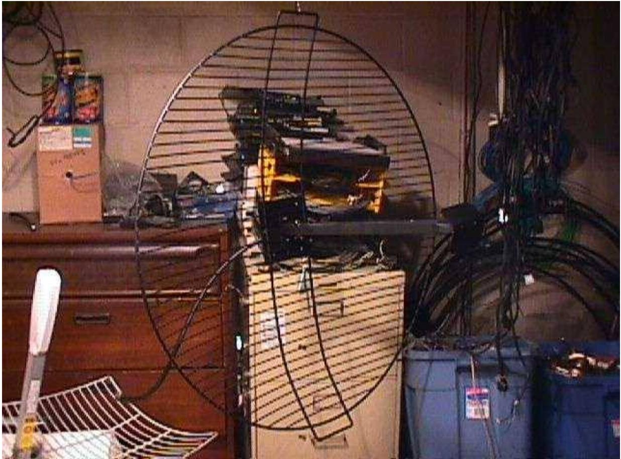
Parabolic antenna reflector used for this project. It's a Lance Industries Model 2536. This 36-inch diameter dish was originally designed for the 2.5–2.7 GHz MMDS band. The gain is approximately 26 dBi and the 3 dB beamwidth is 10 degrees. The focal length is 18-inches.
