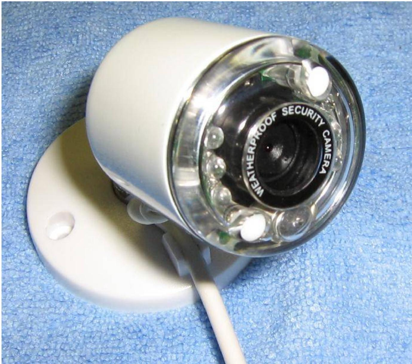
Closeup of the video camera. It is completely sealed inside a fairly weatherproof package. Six infrared LEDs are used for illumination when operating in the dark. The addition of more infrared LEDs with some type of focusing system will greatly increase the "night vision" performance of the camera.
