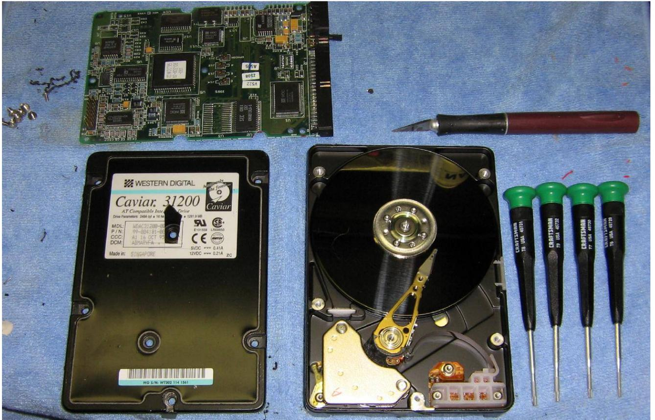
Take the hard drives apart using Torx screwdrivers and an X-acto knife. Save the controller PC board as it is a good source of surface mount components.
