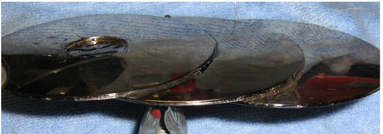
Here are three sandwiched dual-platters epoxied together. Each one overlaps, covering the center hole on the platters underneath it.
