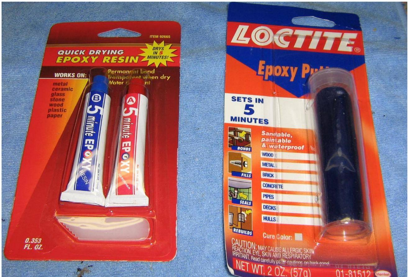
Some of the two-part epoxy resins and putties used for this test. Use the epoxy resin (left) to sandwich two disk platters together for greater strength, then use the epoxy putty to hold the improvised armor in the location you need.
