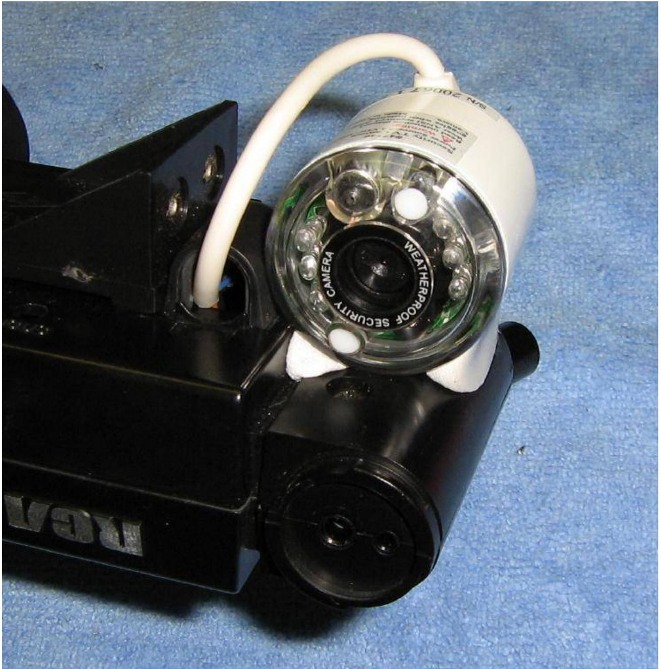
Epoxy the camera to a suitable location on the outside of the **Portable Video Camera Viewer**. Be sure it is pointed in the right direction and "right-side" up – test this ahead of time! Also be sure no screws or adjustment holes are covered up.
