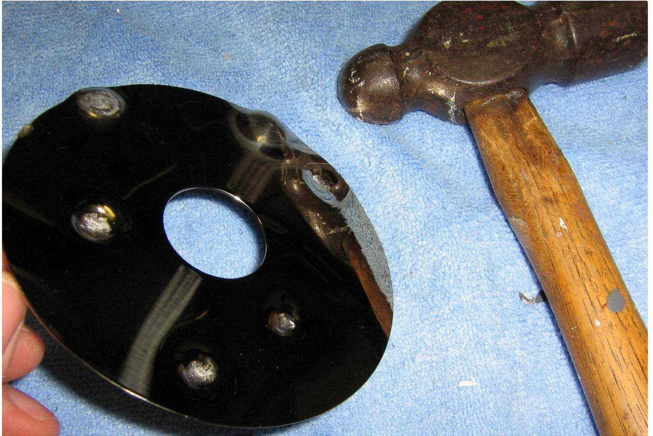
Initial strength test using a ball peen hammer. The individual drive platters appear to be very light (0.5 oz) aluminum discs with some sort of coating. Maybe it's the coating that gives them strength?
