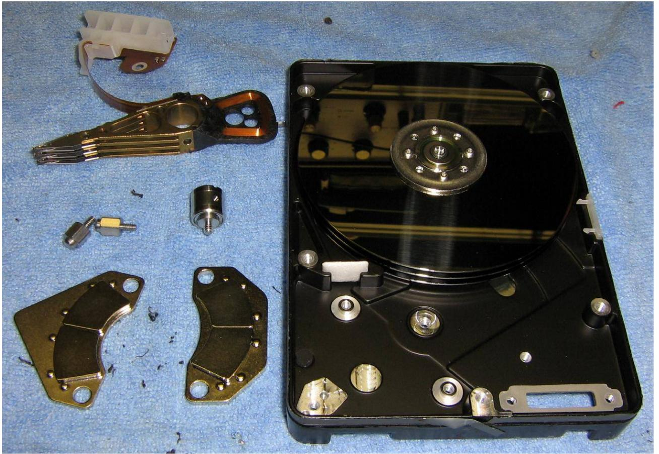
Remove the rest of the mechanical pieces. The magnets on the lower-left are very powerful and can be useful in other projects.
