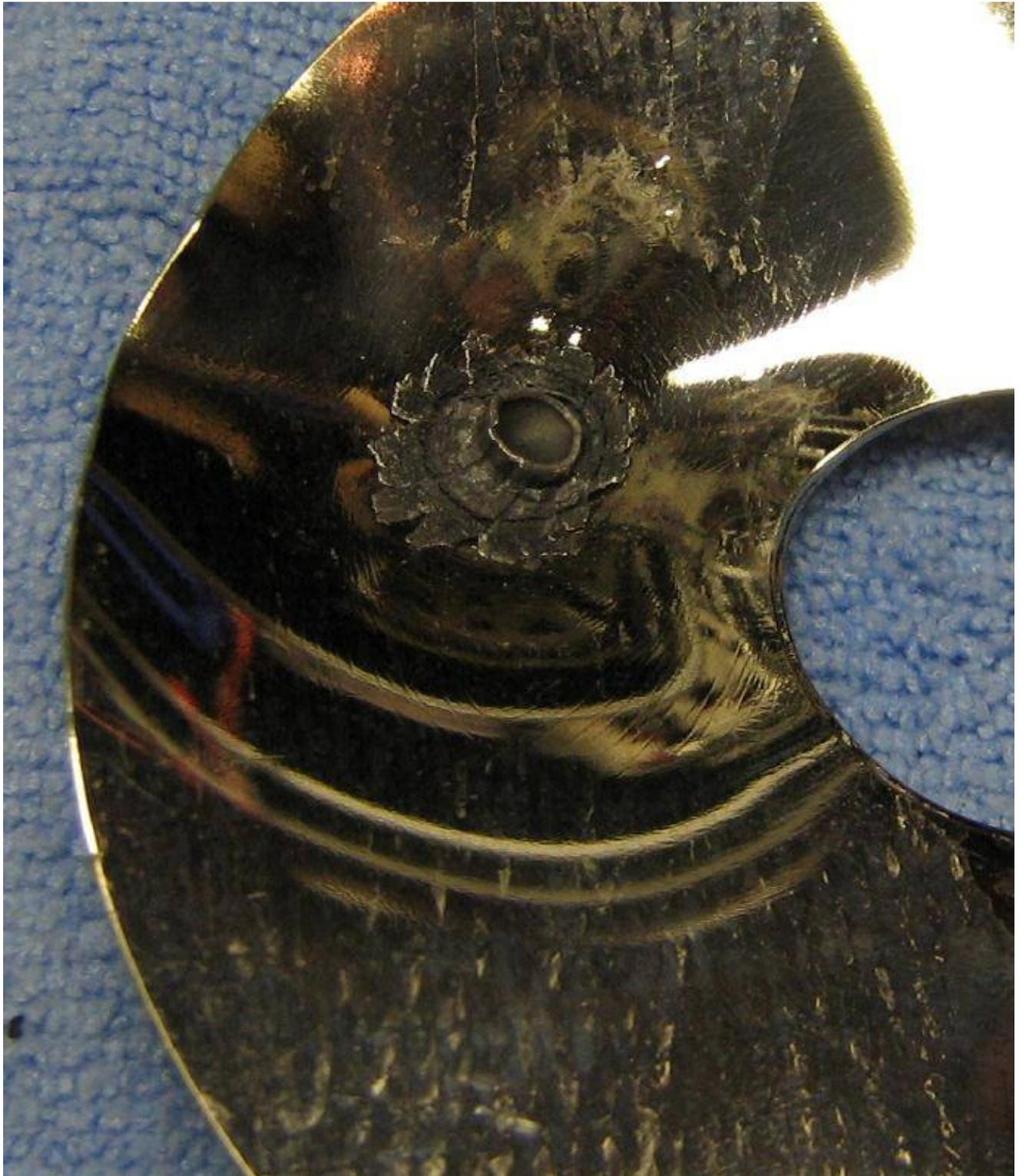
Dual hard drive platters epoxied together – .22 LR. Stopped completely.
