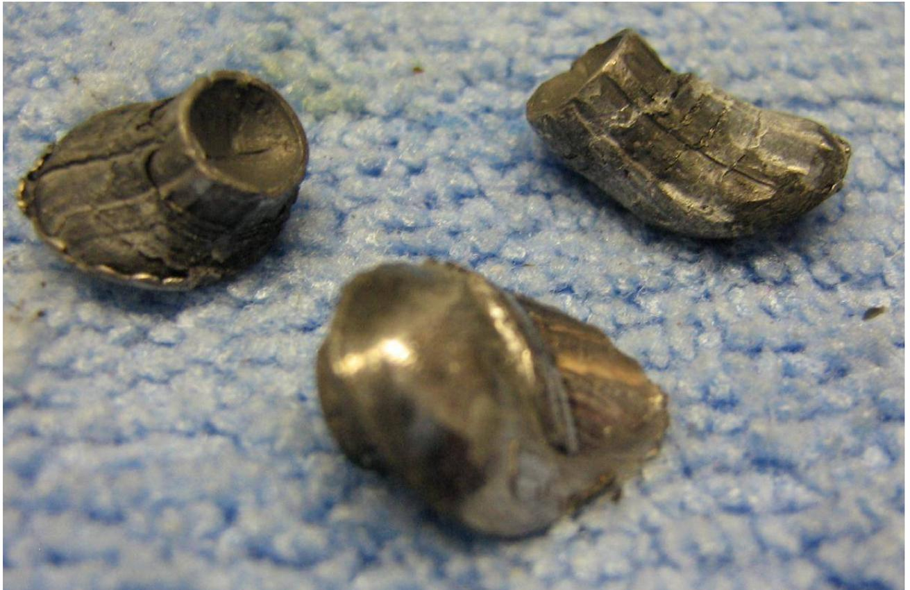
The heavy leather gloves and dual hard drive platter combination could catch the .22 LR bullets.
