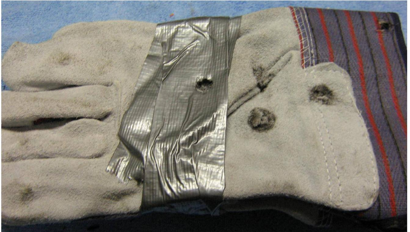
A different test with the dual hard drive platters behind a pair of heavy leather gloves – .45 Colt went straight through. The idea is that thick leather can be used to reduce or even prevent any flesh burns from IEDs.
