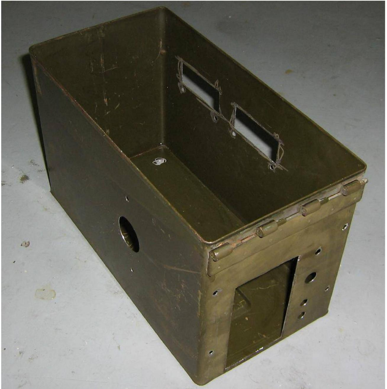
Project case overview. It's an old ammo box, as usual. The two large rectangular holes are for the meter's display and the large 1.25-inch hole (left side) is for a RJ-11 wallplate. The large cutout on the front is for an outlet box.
