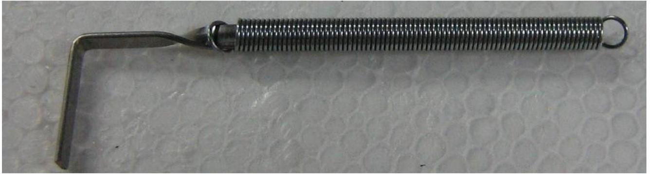
Push a small-diameter spring onto the shortened tension wrench handle. The spring used for this particular wrench is 2-inches long with a 3/16-inch inside diameter. It fits the wrench perfectly. You'll want to purchase a vast assortment of different spring lengths and spring tensions to experiment with.
