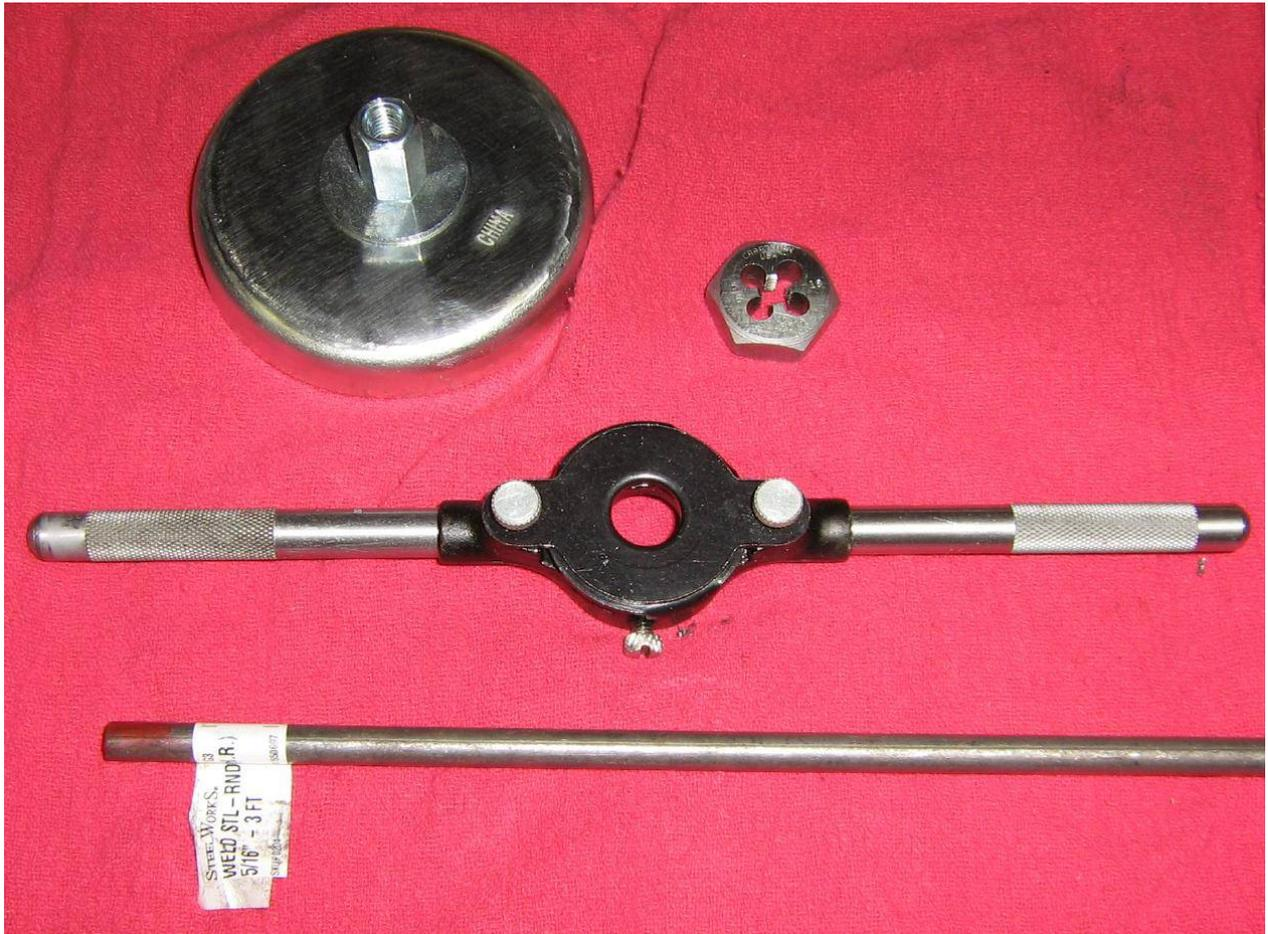
Next, get a six inch long piece of 5/16-inch diameter steel rod and a 5/16-18 thread die. You'll need to thread one end of the steel rod to screw inside the coupling nut.
