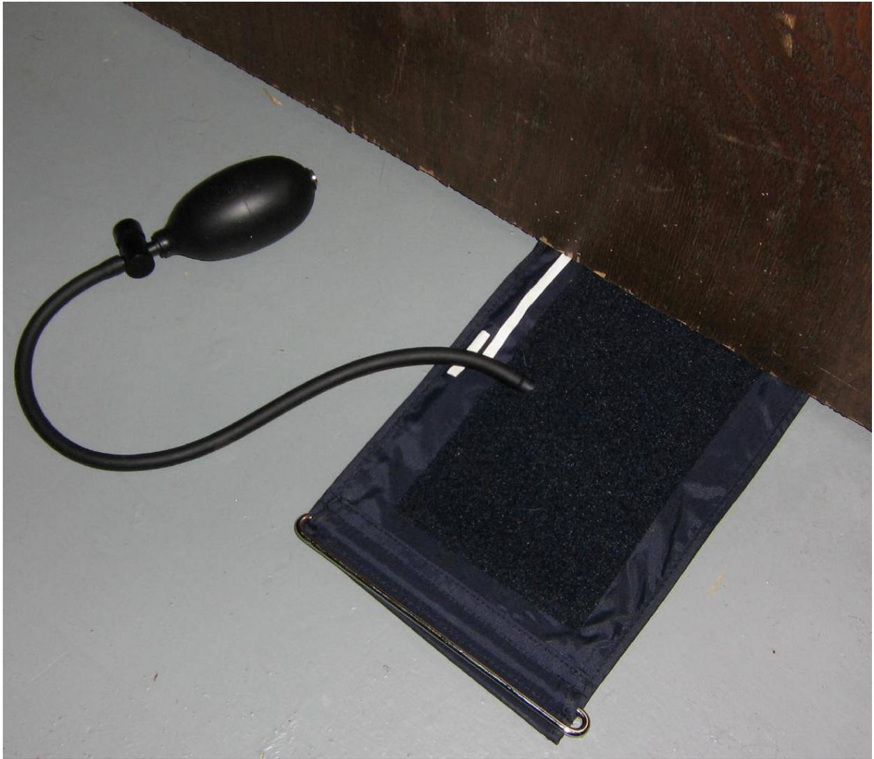
To use it, slide it underneath the door to be lifted. It should be located *away* from the hinge side for maximum "upwards" pressure on the door.
