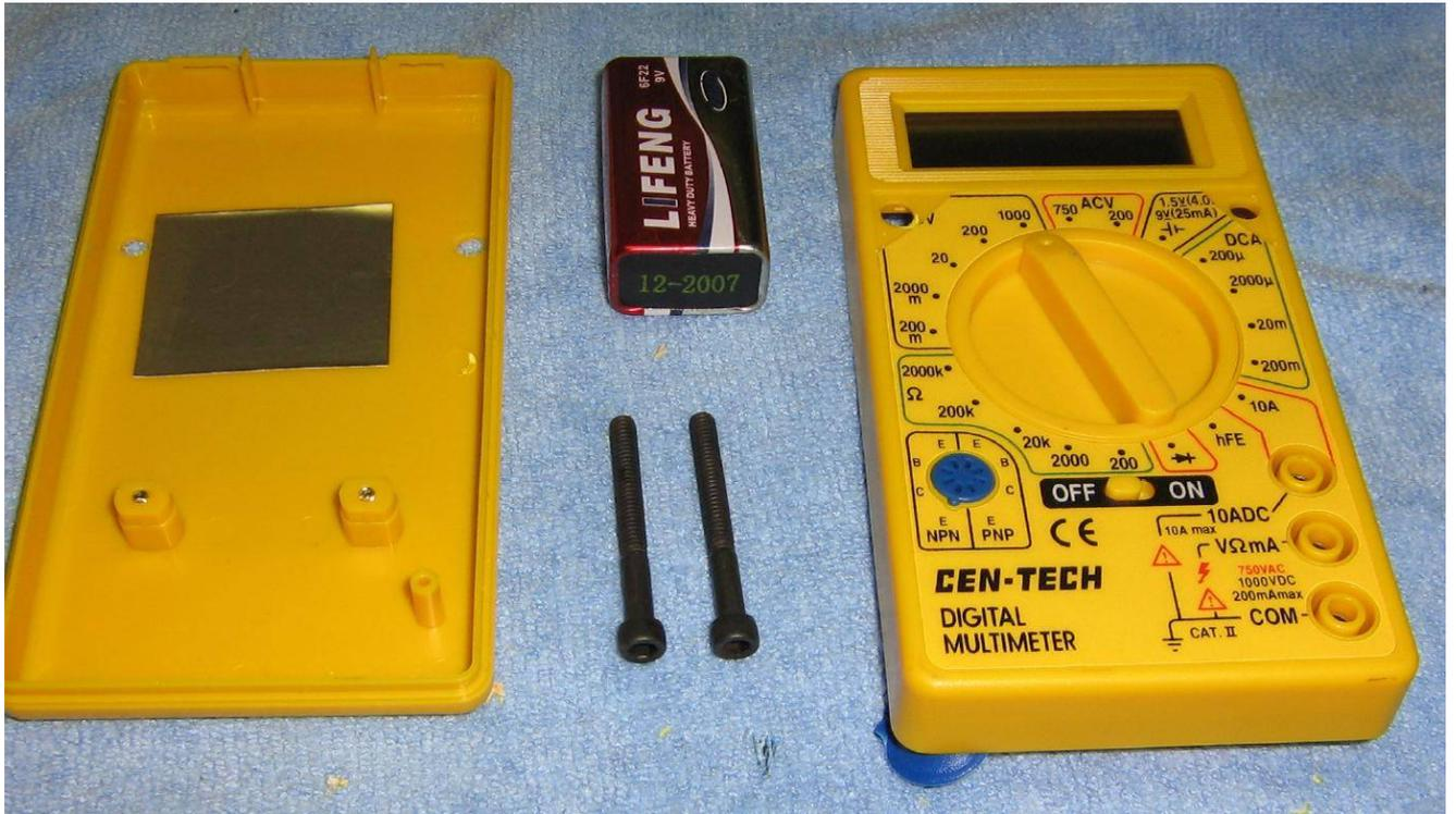
Preparing the digital multimeters. Two 3/16-inch holes are drilled through both plastic covers. They will be mounted to the case using two 1.5-inch long #8 screws and locking hardware. They'll need to be removable to replace the internal 9 volt batteries.
