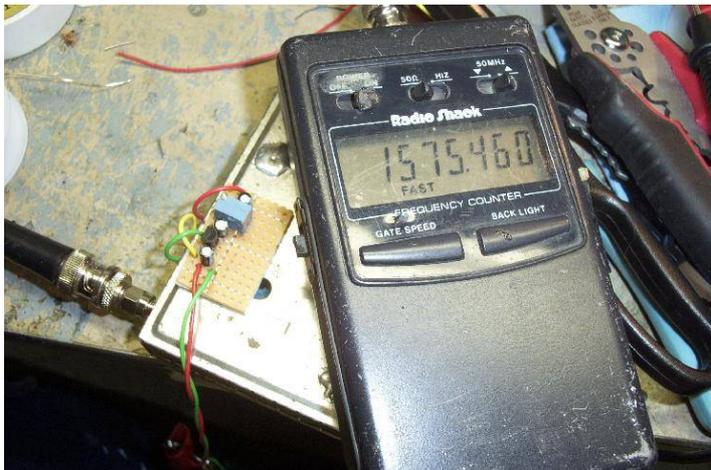
Test setup showing the completed voltage regulator and potentiometer control board mounted to the tuner with double-sided tape. The frequency counter is reading "1575.46 MHz".
