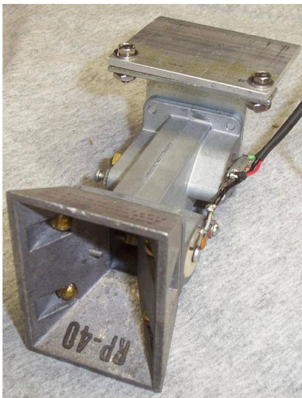
Inside the horn antenna. Be sure to use brass or stainless steel hardware for mounting the horn.
