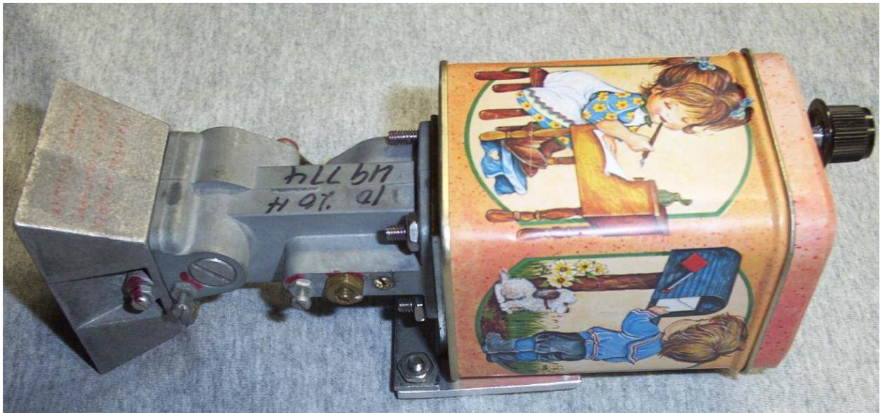
Completed doppler stethoscope. Volume potentiometer has a built-in on/off control. Try to pick a cookie tin that isn't... ahh... so gay.
