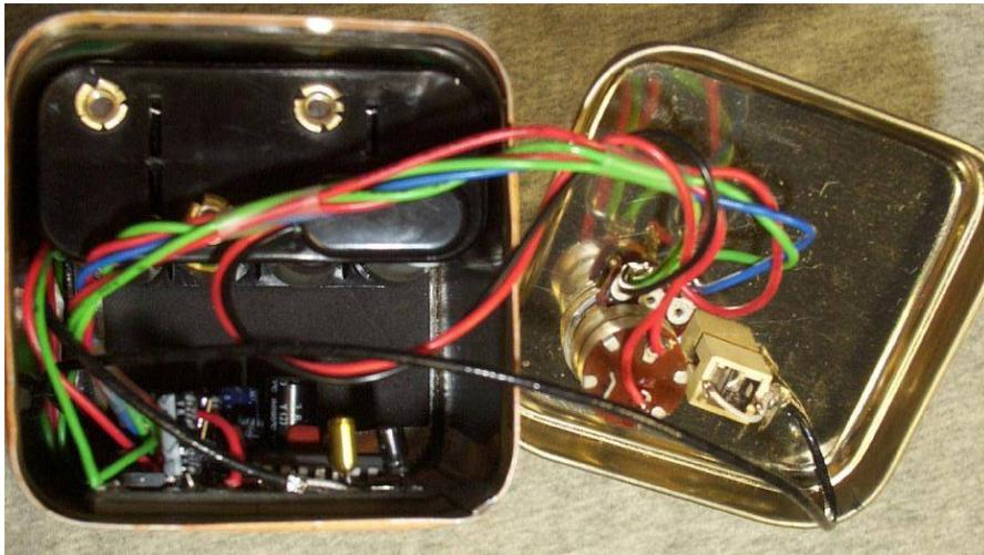
Inside the cookie tin case on the completed doppler stethoscope. A piece of art foam is on the bottom of the tin to protect the battery pack.
