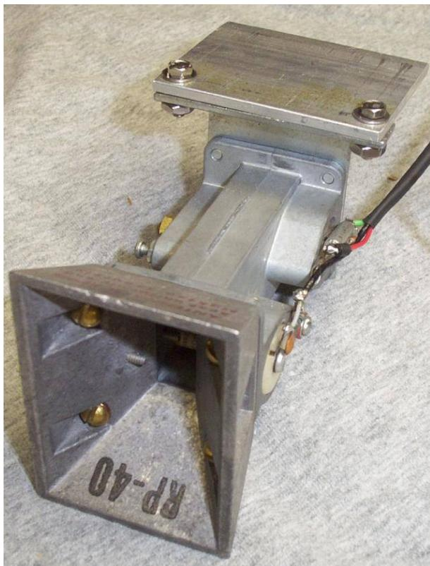
Inside the horn antenna. Be sure to use brass or stainless steel hardware for mounting the horn.
