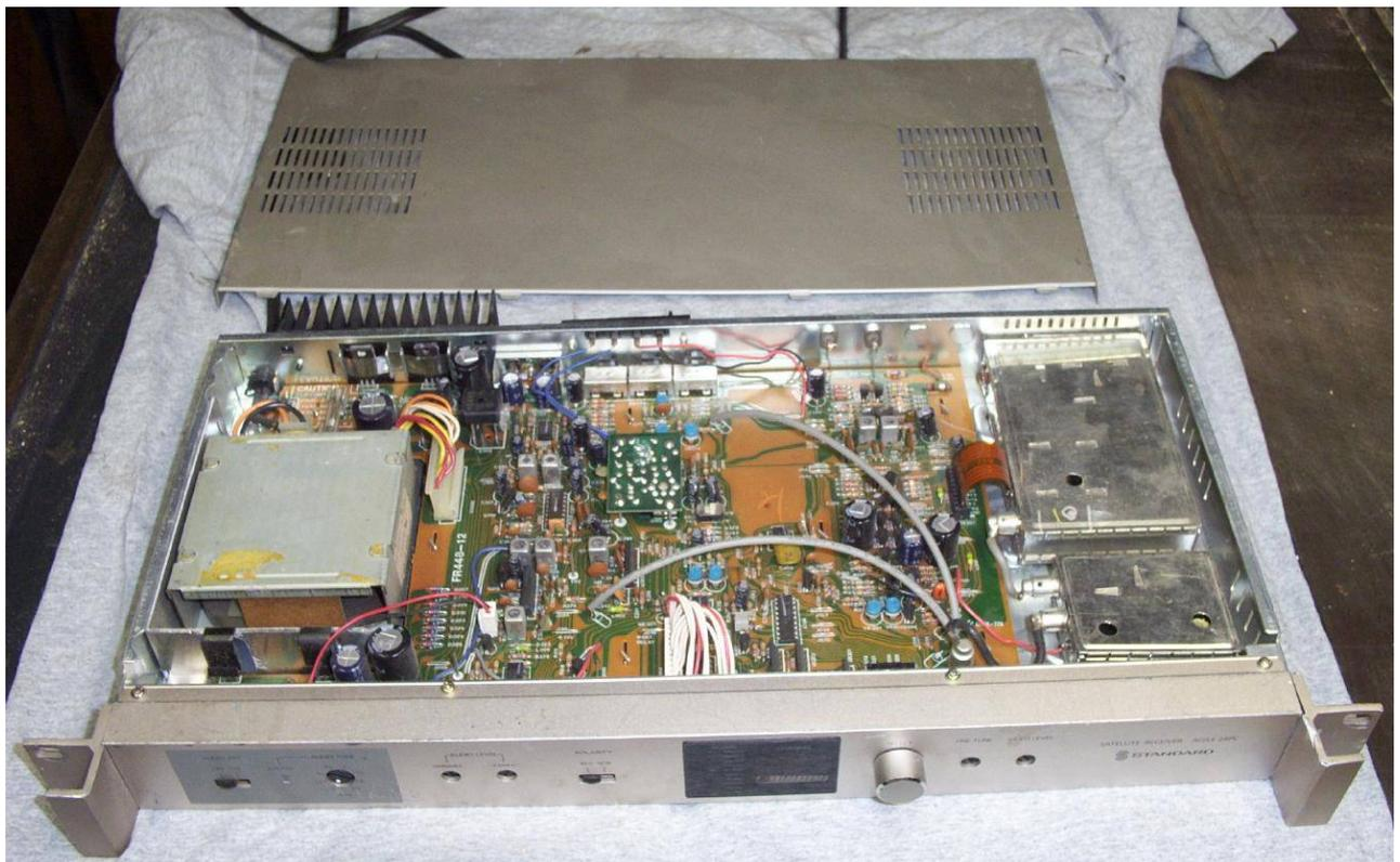
Overview of the satellite receiver used for this project. It is a rack-mount "Standard Satellite Receiver, Agile 24PC". The power supply is on the left, the channel control and demodulator section is in the middle, and the tuner is big silver box on the right.
