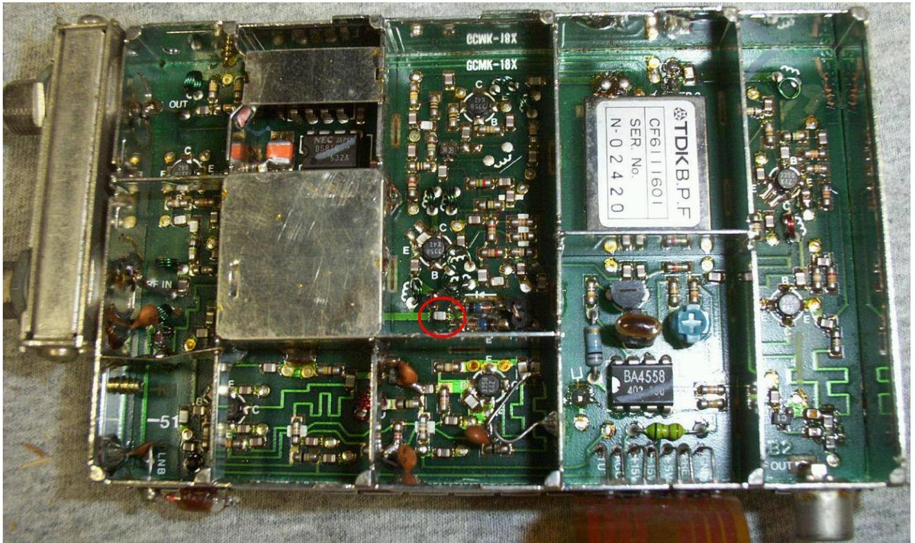
Inside view of an unmodified satellite tuner. 950 – 1,450 MHz RF input is on the left. Under the shielded box are the local oscillator components. Next to that, the section with the two back-to-back diodes is where the RF and LO signals are mixed to form the new 70 MHz IF signal. The box with the "TDK" logo on it is a bandpass filter for the IF. The IF signal is then further amplified and sent to the RCA jack on the bottom right.
