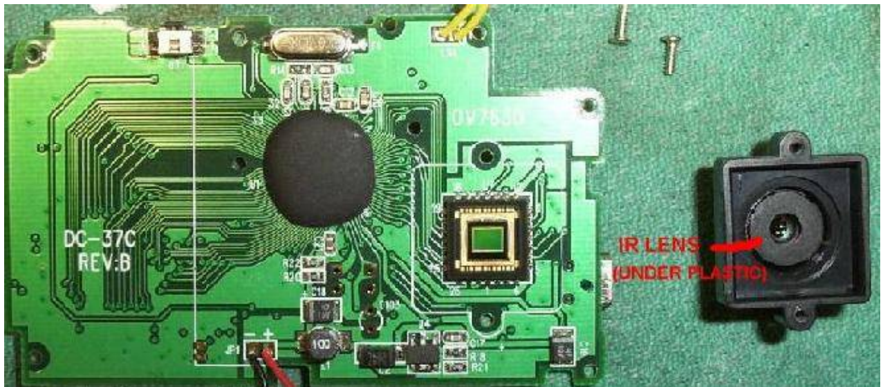
Close up picture of the camera's front PC board with the plastic lens assembly removed. Be sure to not get any dust on the CMOS imager's window.
