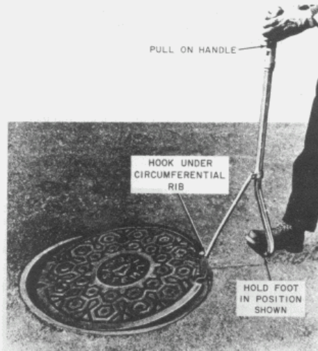
Fig. 30—Unseating Cover With PTS-49 Manhole Cover Lifter
