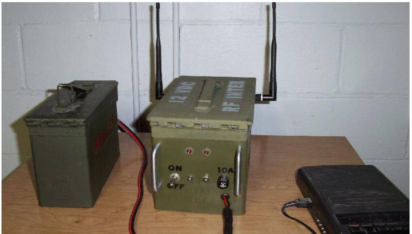
Testing setup. The green ammo box on the left is a large 12 volt lead-acid battery. The jammer is in the middle and the "victim" tape recorder is on the right. The effective jamming radius of this setup was only about a meter. More RF power output and/or directional antennas will increase the range.
