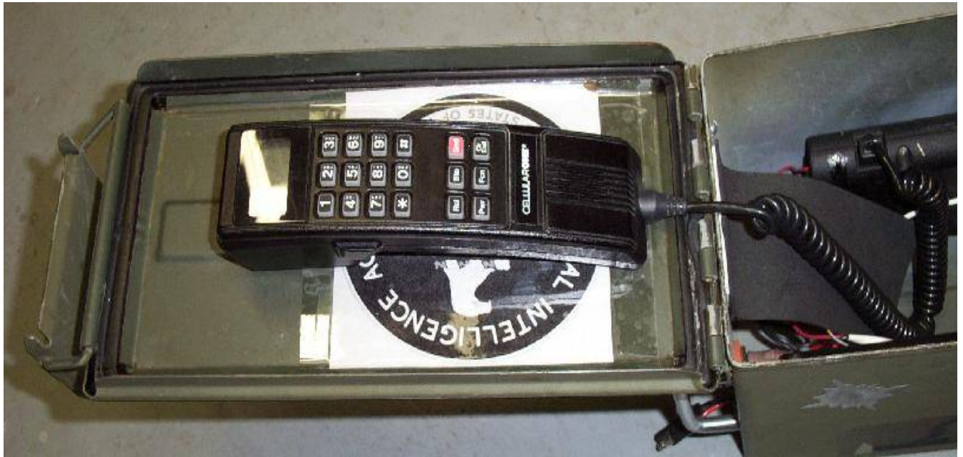
Handset picture. The handset is bolted to the ammo box's cover. Be sure it doesn't pinch the cable when closing. A large CIA logo is underneath the handset.
