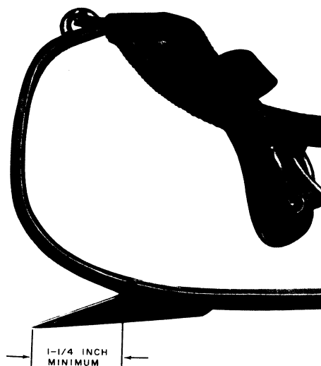
Fig. 21—Gaff Sharpened to Minimum Length
