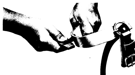
Fig. 18—Removing Burrs From Bottom Cutting Edge
