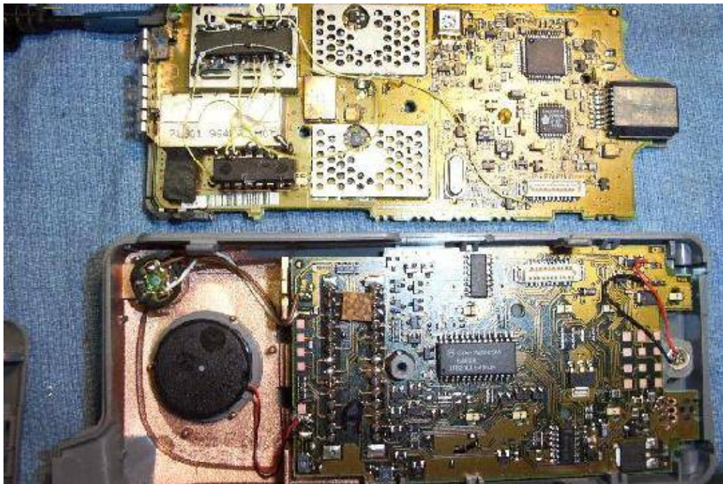
Internal view of a "bugged" Motorola TeleTac 250.
