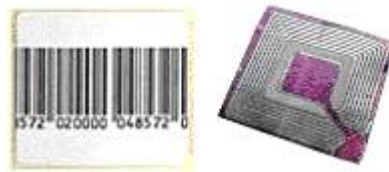
Figure 4. A RF barcode sticker that functions as a security device, complete with a tank circuit on its back. The tag can be made useless by breaking the circuit, for instance by slicing through the sticker with a razorblade or Xacto knife.
