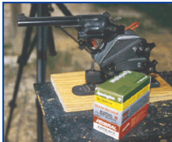
Ransom Rest testing is the only way to really proof revolver and ammo. (Below): This vintage 5-screw K-38 is happiest when digesting factory wadcutters.
