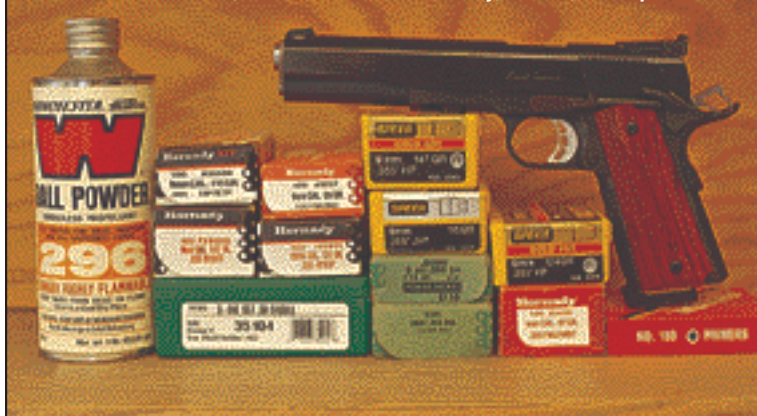
Components used in handloading the .38 Casull: Winchester 296 powder, Federal #155 Primers, and bullets from Hornady, Sierra, and Speer.
