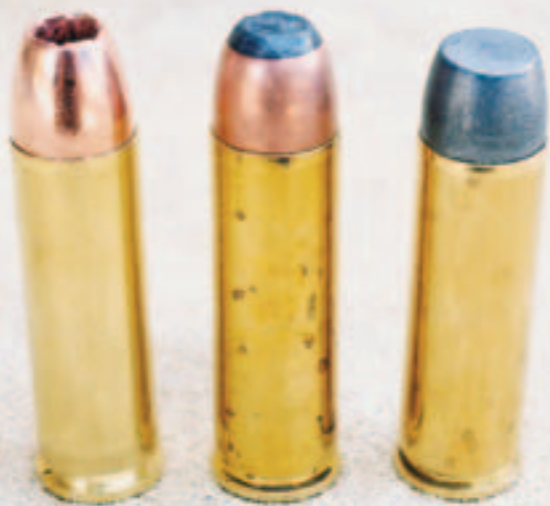
.500 S&W loads tested included (left to right) a 275-grain Barnes X-Bullet at 1,665 fps, a 400-grain JSP at 1,675 fps and a 440-grain hard cast flat point at 1,625 fps.
