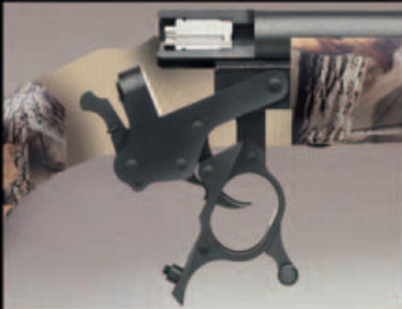
Omega's unique breech mechanism has only four moving parts. Simply pull down the trigger guard and the pivoting action drops the breech block clear of the breech face. Slip in a 209 primer and you're primed.
