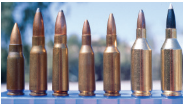
The evolving super shorts: Left to right: 7.92x33 Kurz; 308x1.5; 7.62x39; 5.6x39; 6mm PPC; .223 WSSM and .243 WSSM.
