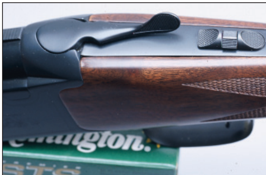
Above: Combo safety/barrel selector makes choke selection fast and easy. Below: Generous checkering graces the wrist of the 332.
