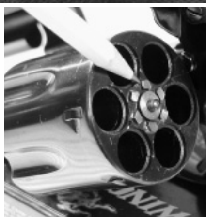
Below (left-right): Rimfire chamber counterbores are often damaged. Gas cutting above barrel cylinder gap is obvious. Cylinder ratchets deserve careful inspection. Standing breech and exposed hand on Ruger SA revolver. Note how recoil has imprinted the ratchets around the base-pin hole.
