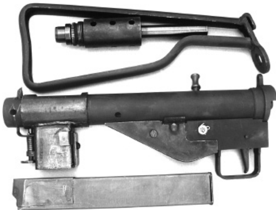
This Mark II Sten shows how compactly it could be packaged for air-drop. It can be assembled and made ready to fire in 20 seconds.
