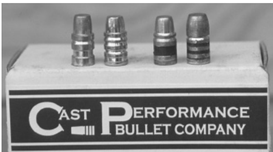
Above: Think you need jacketed bullets for excellent accuracy in .357 Magnums? Try CPBC's 187 grain FNGC. Below: Cast bullets used in the .357 Magnum include Lyman's #358429, #358156, BRP's 155 SWC-GC, and Cast Performance Bullet Company's 187FP-GC.
