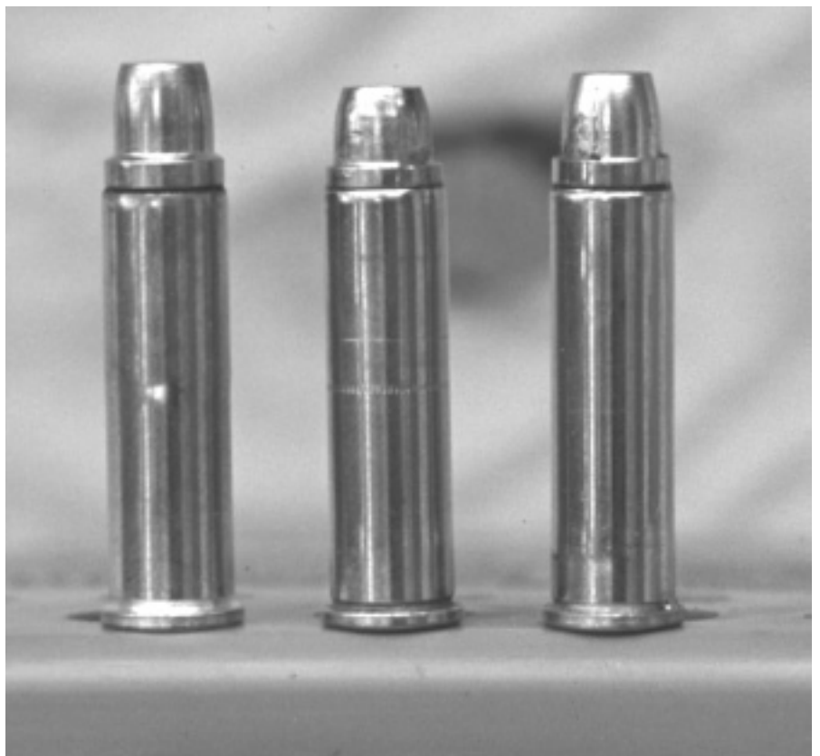
Note the difference in overall length in the .357 Magnum loads using (L-R) Lyman's #358429 and #358156, RCBS's 38-150KT.
