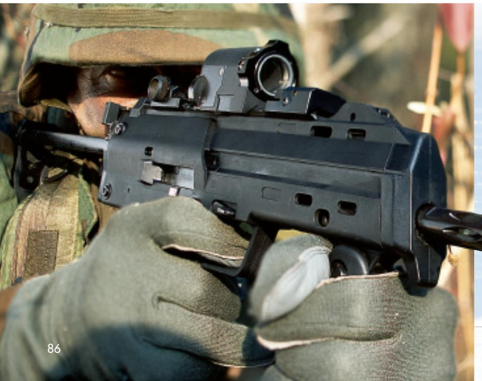
or under low light conditions, from a battery or tritium insert. There are backup open sights in case the optical sight becomes damaged or is removed.
