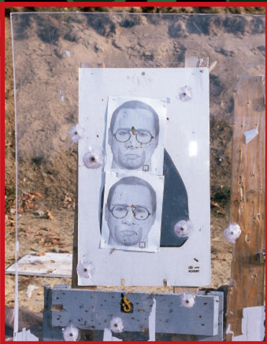
***Glass is very hard on rifle bullets, which are often deflected or fragmented, as seen here. With suitable projectiles the .300 WSM should offer an advantage shooting through glass and other obstacles compared to the .308.***
