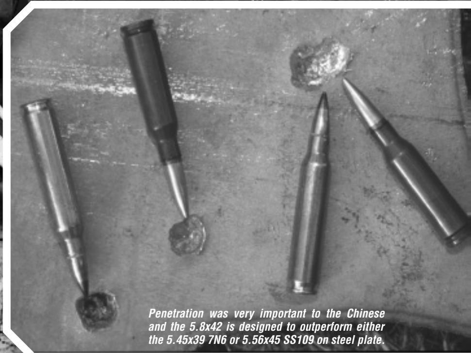
*Penetration was very important to the Chinese and the 5.8x42 is designed to outperform either the 5.45x39 7N6 or 5.56x45 SS109 on steel plate.*
