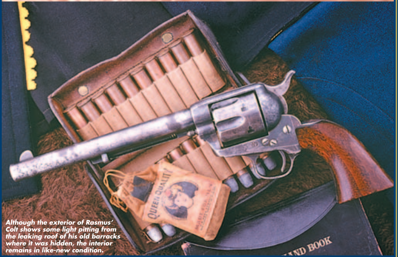
Fearing he would get in trouble for having an army Colt, Rasmus peened out the "US" acceptance stamp on the left side of the frame. He also expertly removed the cartouche from the wooden grip and refinished it as new.
