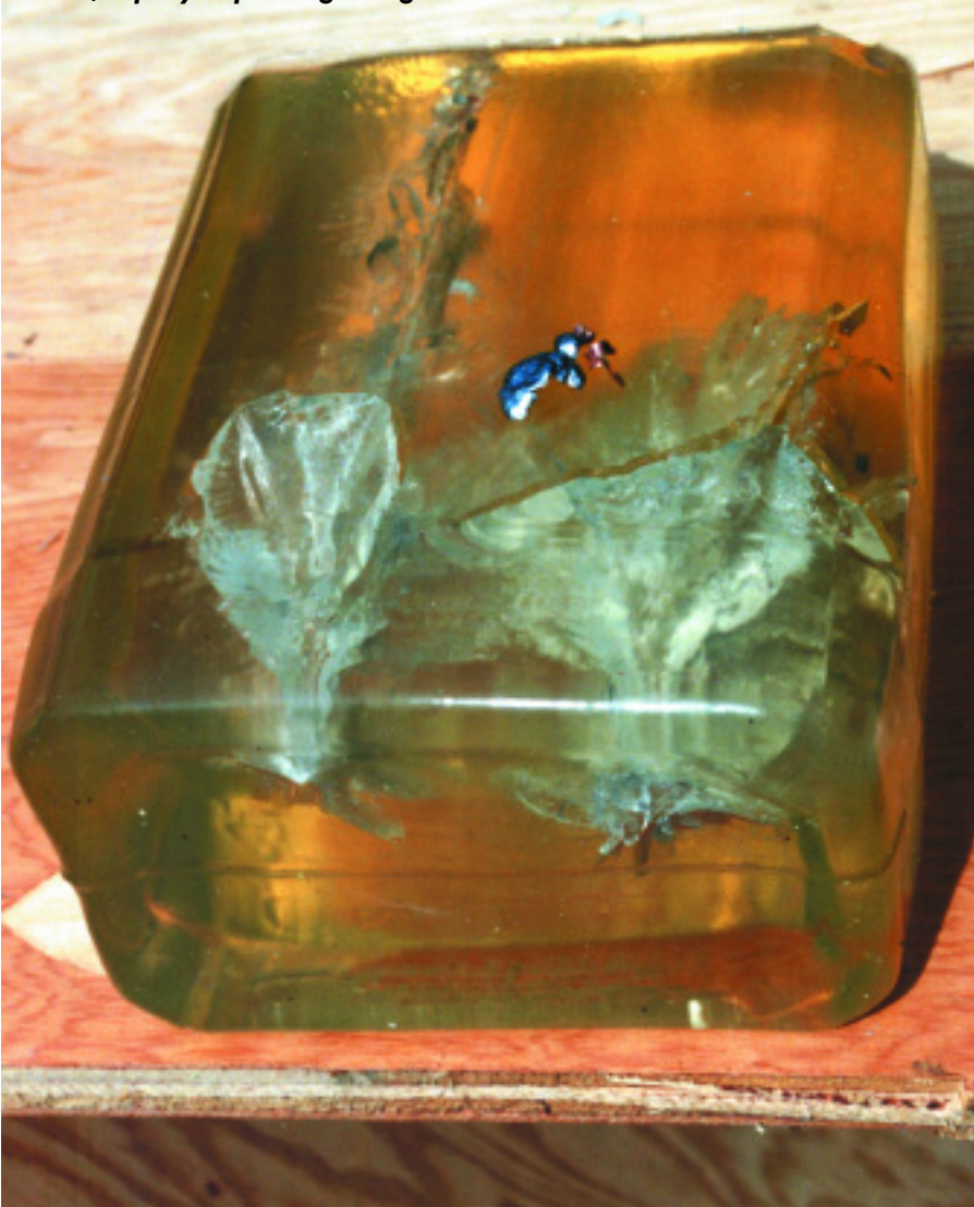
Gelatin block shot with poorly expanding bullet on left, rapidly expanding on right.
