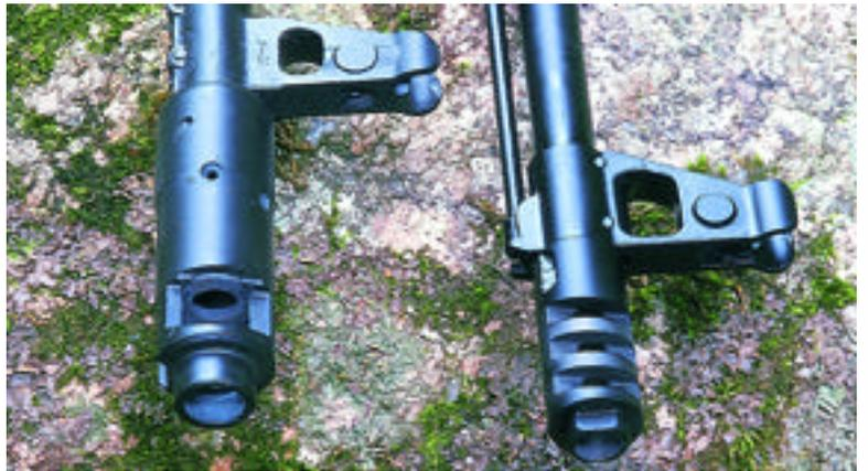
The SA M-7's muzzlebrake (right) is as effective as the Russian AK-103 brake (left), yet produces less flash.
