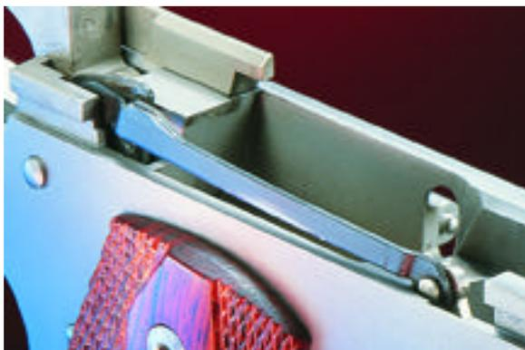
The Para-Ordnance LDA system is a marvel of expert engineering. Shown above are two views of the trigger draw-bar.
