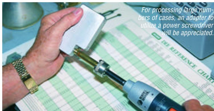
*For processing large numbers of cases, an adapter to utilize a power screwdriver will be appreciated.*
