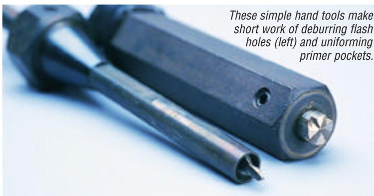
*These simple hand tools make short work of deburring flash holes (left) and uniforming primer pockets.*
