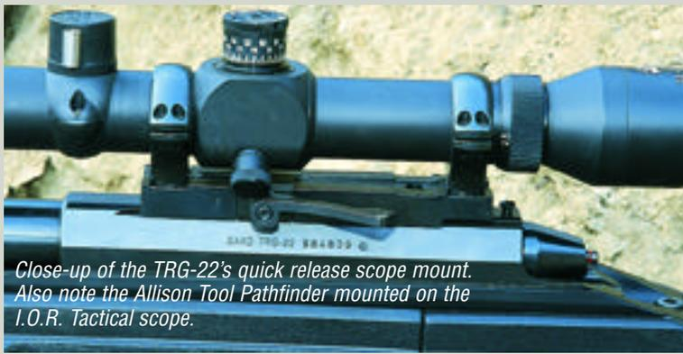
*Close-up of the TRG-22's quick release scope mount. Also note the Allison Tool Pathfinder mounted on the I.O.R. Tactical scope.*
