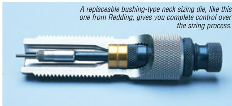
*A replaceable bushing-type neck sizing die, like this one from Redding, gives you complete control over the sizing process.*
