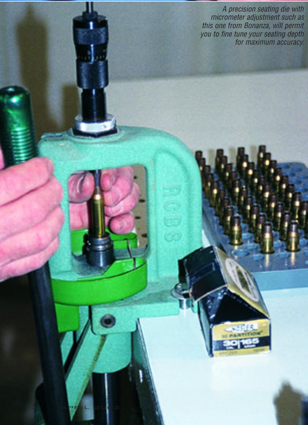
*A precision seating die with micrometer adjustment such as this one from Bonanza, will permit you to fine tune your seating depth for maximum accuracy.*
