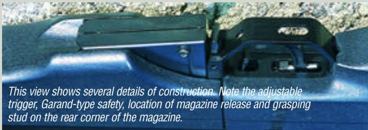
*This view shows several details of construction. Note the adjustable trigger, Garand-type safety, location of magazine release and grasping stud on the rear corner of the magazine.*
