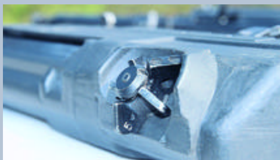
Above: The rear sight is a simple yet novel design that incorporates settings for 200 and 400-700 meters. Below: The muzzle device on the AN-94 is a vast change from the muzzlebrake on the AK-74M.
