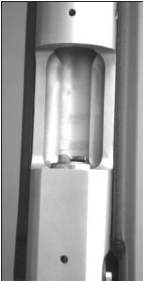
Above: View of the open bolt shows the slot which accepts a No. 209 shotgun primer. Left: The new Savage Model 10ML-II is a handsome rifle built for rugged hunting conditions.
