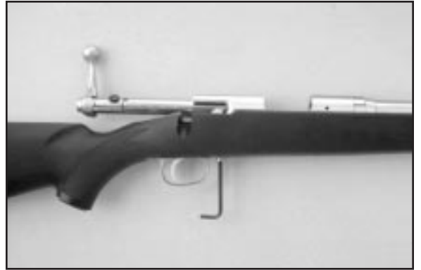
Turning out a single screw with an Allen wrench permits removal of the bolt for access to the breech plug.
