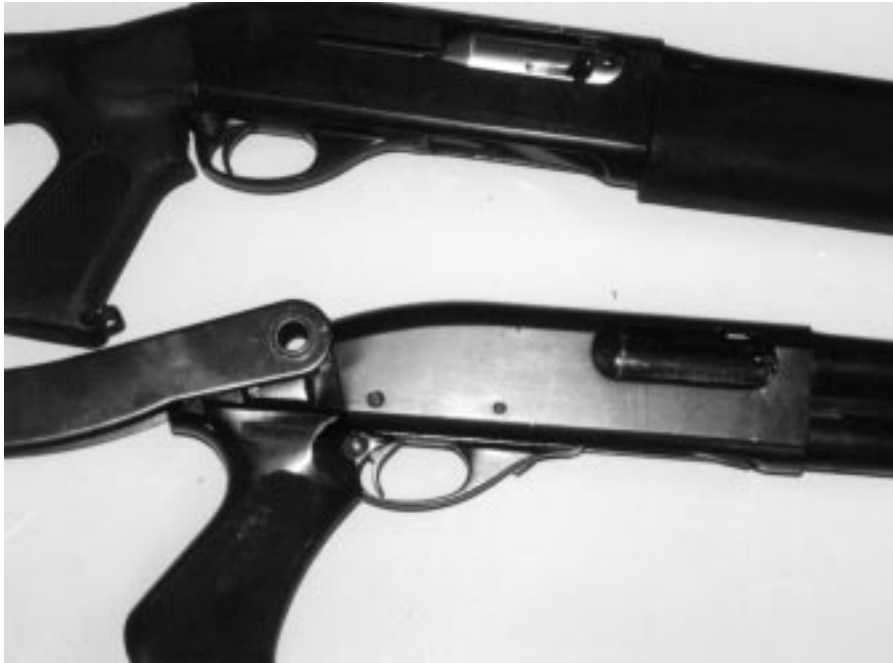
Gas operated auto shotguns, like the Remington 1100 (top) with Choate stock, will always kick distinctly less than comparable pumps like the Remington 870 (below) with Remington's folding stock.
