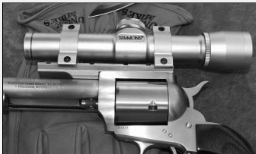
The TSOB scope mount system from SSK comes with three rings, but only two are used on the .41 Magnum.
