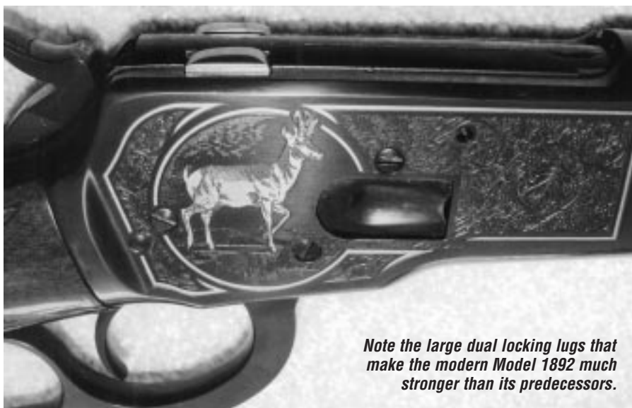
The Model 1892 has a tang safety and rebounding hammer.
