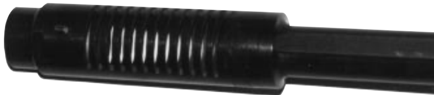
Below: The old Cutts Comp opened the door to reducing shotgun recoil at the muzzle. Long superseded by more efficient devices, they're still better than nothing.
