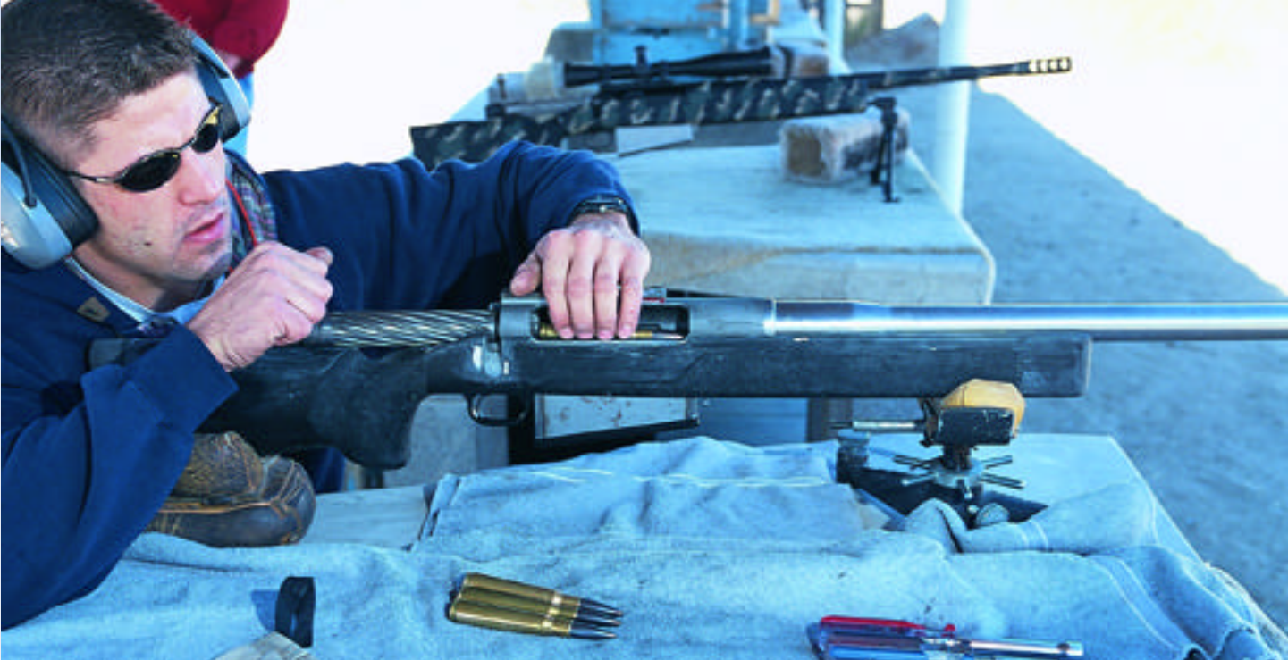
A yet to be finished Robar RC50 is tested for proper function. Notice that no telescope is attached. For these preliminary tests, there is no need to subject a good scope to the pounding recoil of the .50 BMG.
