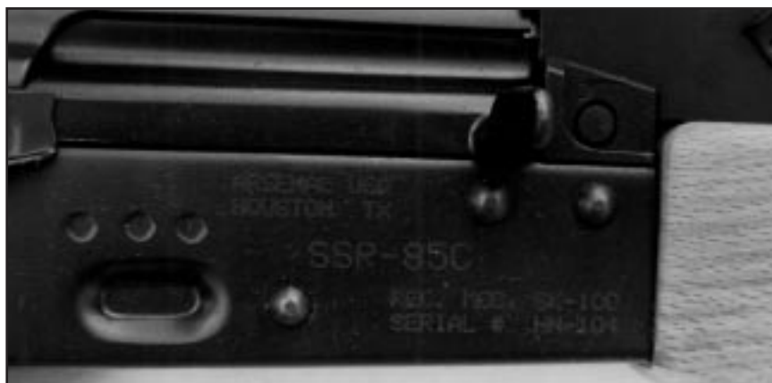
Receiver markings of the SSR-85B and SSR-85C models
