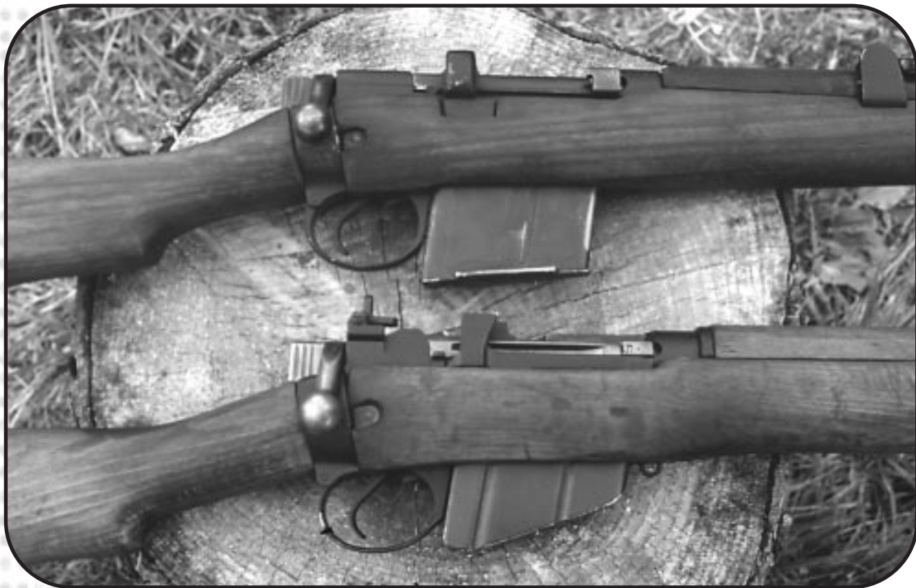
The square looking magazine of the .308 2A1 Enfield differentiates it from its .303 No. 4 brother.
