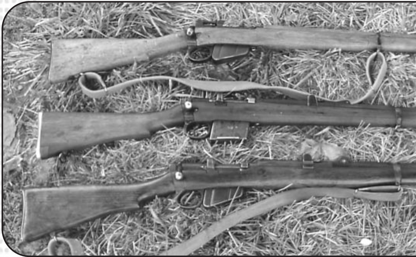
Lee Enfield combat rifles: (top to bottom) .303 No. 4, the Ishapore .308 2A1, and the .303 No.1 Mark III.
