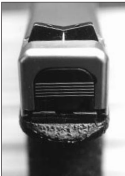
Right: The rear sight of AO Sight Systems' Pro-Express Big Dot Tritium is a shallow V with a vertical tritium stripe. Left: The front sight of the AO Big Dot is 4mm, far larger than the 2.8mm of AO's regular tritium sight.
