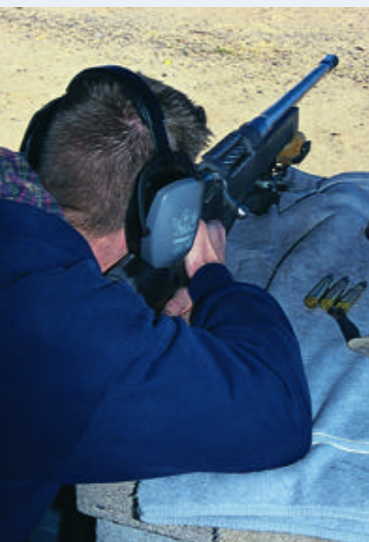
A yet to be finished Robar RC50 is tested for proper function. Notice that no telescope is attached. For these preliminary tests, there is no need to subject a good scope to the pounding recoil of the .50 BMG.
