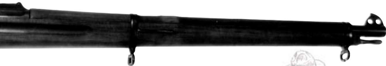
Very early M1903. Notice the rod bayonet and very different front and rear sights.
