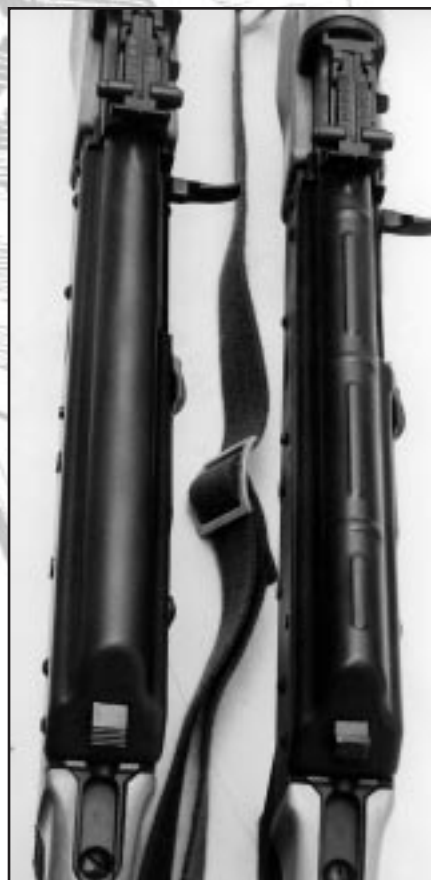
Notice the AK-47-style top cover on the SSR-85C (left) vs. ribbed AKM-type cover of the SSR-85B.
