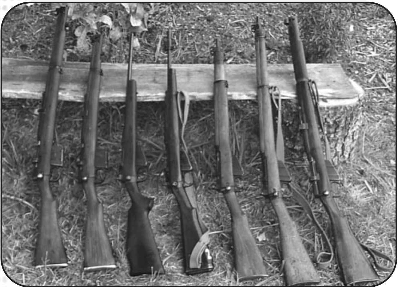
Left to right: as issued .308 2A1; cut-down .308 2A1; cut-down .303 No.4 with synthetic stock; as-issued .303 No.5 Jungle Carbine; cut down .303 No.4; as issued .303 No.4; No.2 MK III
