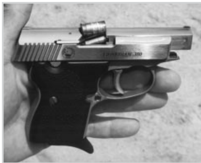
Above and Below: Typical last-shot malfunction with Remington... and—the only time it happened before the last shot—Federal.
