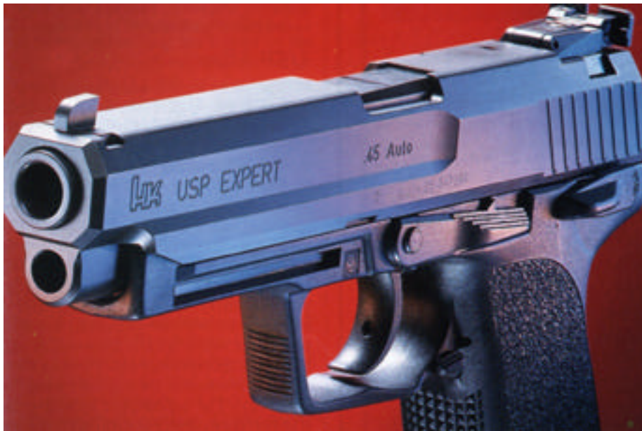
The Expert comes only in .45 ACP and uses a longer slide with a distinctive profile than others in the USP family. Like the USP Tactical, the Expert features a match grade trigger with an overtravel stop. At right, an underside view of the trigger guard with the press-down-to-release ambi mag catch.
