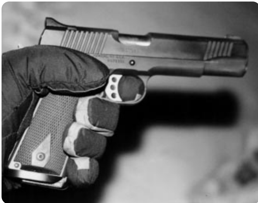
With ambi safety, newest Kimber worked well southpaw, and with good "street trigger," was safe in a gloved hand.
