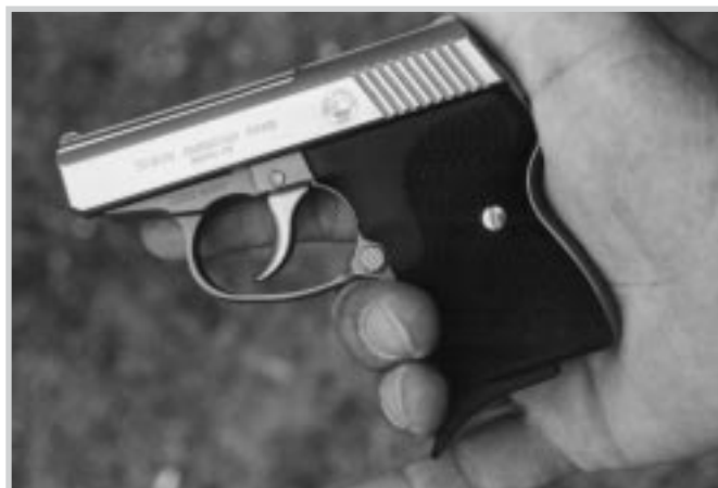
Pistol comes with flush bottom magazine, which allows 1.5 finger wraparound... and another with finger extension, allowing two whole fingers purchase.
