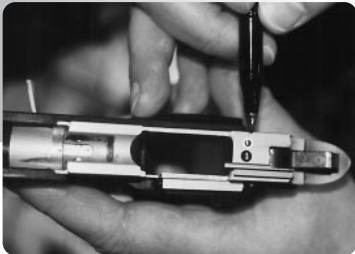
Pen points to Schwartz/Sirkis firing-pin safety interface as it projects from a stainless Kimber's frame...
