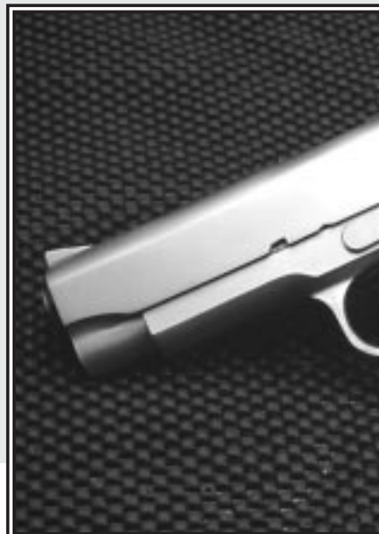
Two views of a "Swensonized" Colt Gold Cup. The slide and barrel have been shortened, and the pistol features S&W K-sights, Swenson's signature hard-chrome finish and 60 degree checkering. The latter is very unusual for a Swenson gun.
