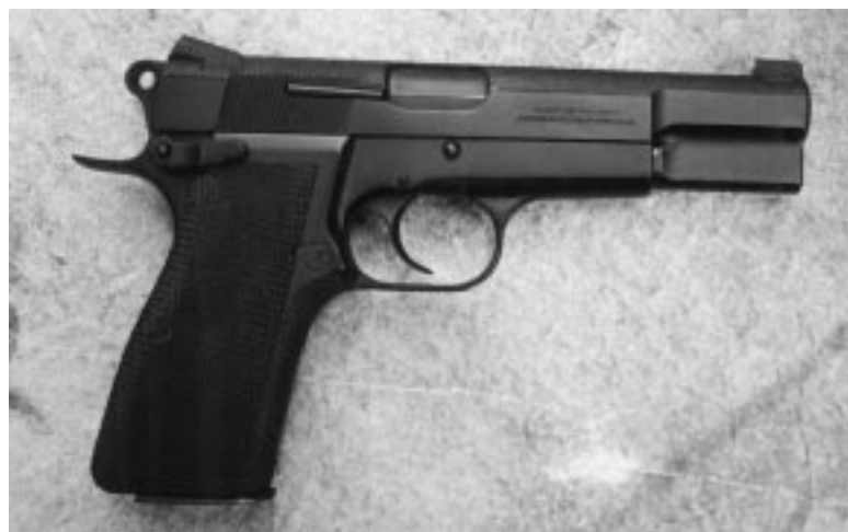
While the Browning P-35 is an excellent pistol out of the box, it can be improved. This example shows Novak sights, an extended backstrap, a wide trigger, and texturing of grip and sighting surfaces.
