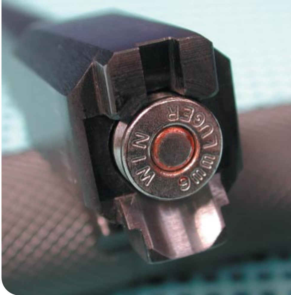
The case head is well-supported and the integral ramp and barrel show top quality machine work.
