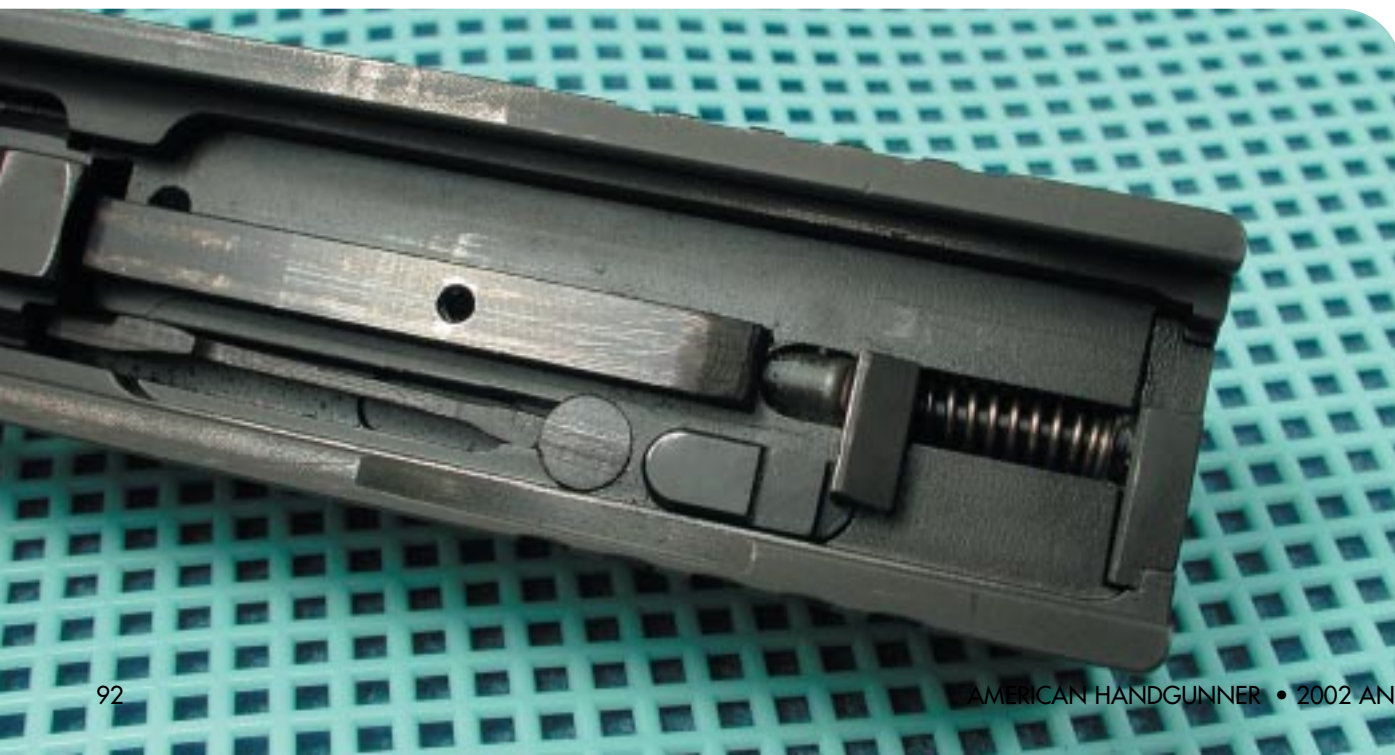
The interior of the slide shows first-rate machining in this all-steel forging.
