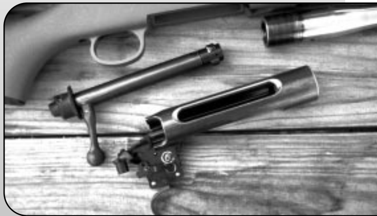
Components of the Remington 710 include a steel receiver; synthetic insert to house the trigger mechanism and act as a bolt guide; three-lug bolt; synthetic stock; and the barrel is compression-fitted into the front receiver.
