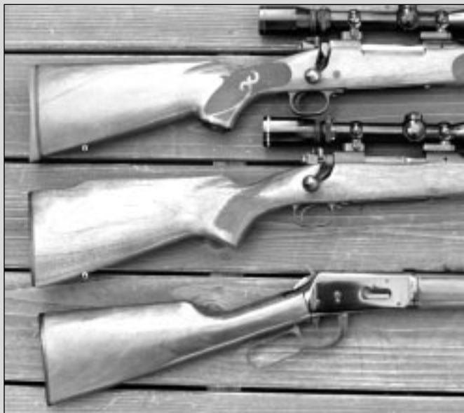
Stocks have become straighter, with less drop at comb and heel, as is illustrated by Winchester rifles spanning three eras. Top, current Model 70 Featherweight; center, Model 70 from the early 1960s; bottom, Model 94.
