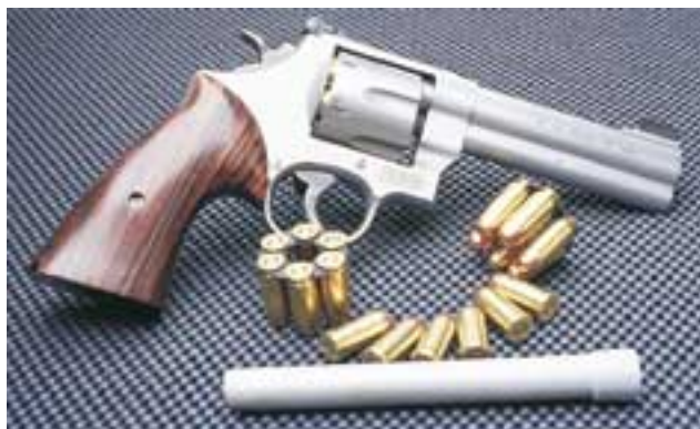
The aluminium rod is a tool from SSK to pry those stinker .45 ACP cases from moon clips.
