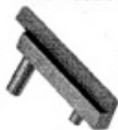
#315 / KING'S N.M. CUSTOM SEAR SPRING. Use with lightweight trigger for correct trigger jobs. No need for special hammer and sear to keep hammer cocked when loading or firing. Engages disconnector and trigger stirrup. Lets you use government model hammers and sears for trigger jobs. $6.00
