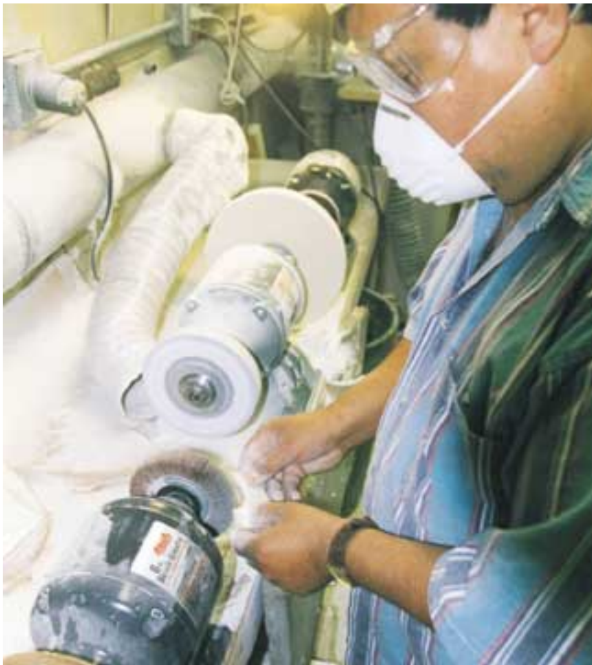
A gripsmith in Eagle's Illinois facility demonstrates how to polish with the latest in OSHA-approved ventilation equipment.
