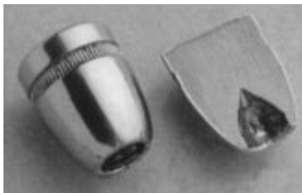
Hollow cavity projectiles can fill with sheetrock and behave like FMJ bullets (right).
