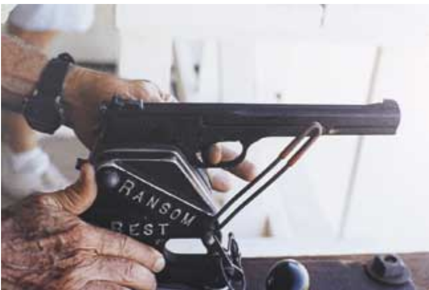
A Model 41 goes into a Ransom Rest. This device is the arbiter of accuracy, the Independent Counsel of bullseyes. Hamilton asserts that any properly fitted 1911 can shoot 1.5" at 50 yards from one of these babies.
