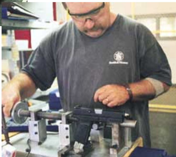
Herb Belin (left) inspects a robotic measuring device checking a frame for correct tolerances. Every S&W pistol is checked for trigger pull (below) with a special computerized measurer.
