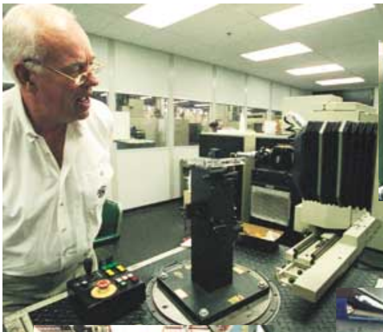
Herb Belin (left) inspects a robotic measuring device checking a frame for correct tolerances. Every S&W pistol is checked for trigger pull (below) with a special computerized measurer.
