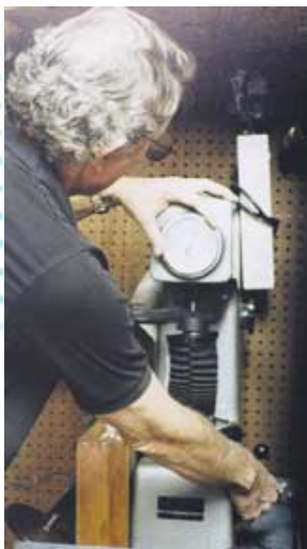
Alex Hamilton with a Rockwell testing machine, checking hardness on a Springfield Armory slide. It passed.
