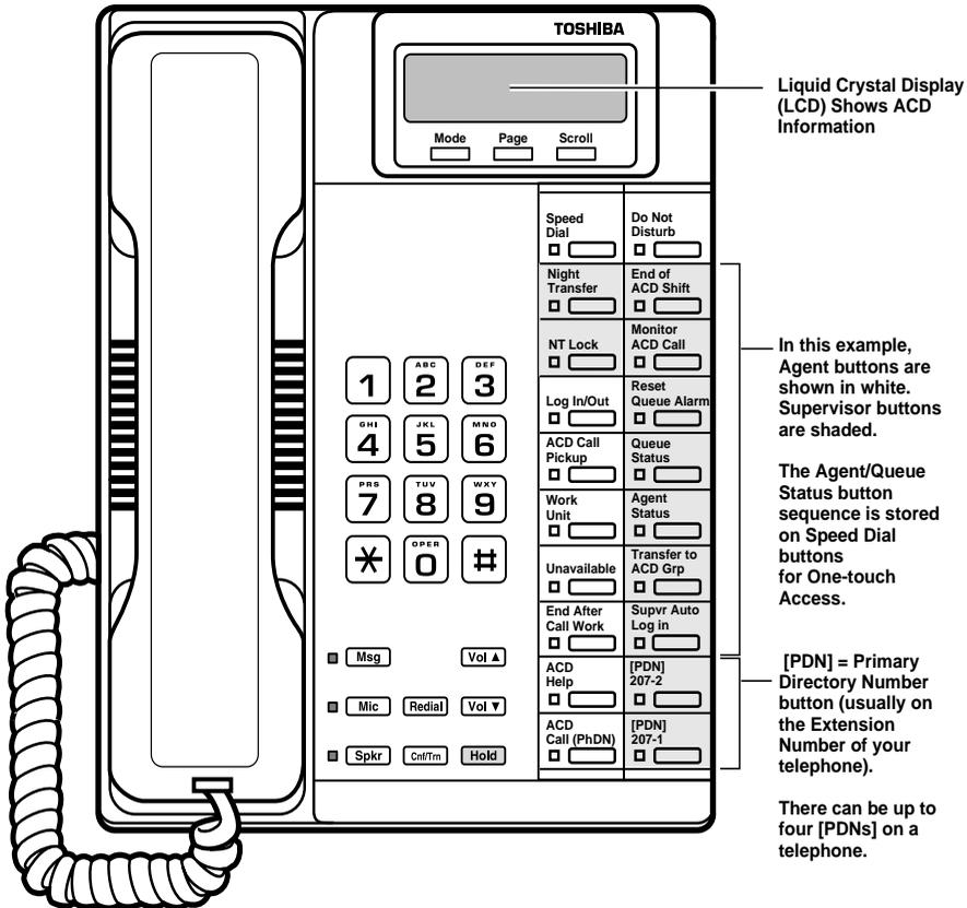
**Figure 1** ACD Supervisor Digital LCD Telephone
