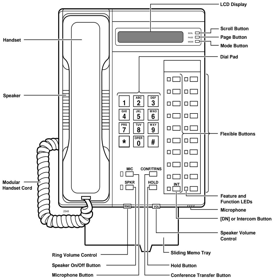
Figure 1 20-Button Electronic Key Telephone with LCD
