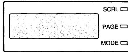
The Liquid Crystal Display (LCD) digital telephone is a 20-button speakerphone with the LCD as an additional feature. All features and functions of the LCD telephone, exclusive of the display itself, perform exactly like the non-LCD 20-button telephone.
