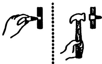
For plaster, plasterboard, cinder block, or brick surfaces, drill a 3/16" hole at each mark and insert an anchor into each of the holes. Gently tap each anchor with a hammer until it is flush with the surface. Screw the screws partially into the anchors, remove them, hang the tabs on the screws, and then tighten the screws.
