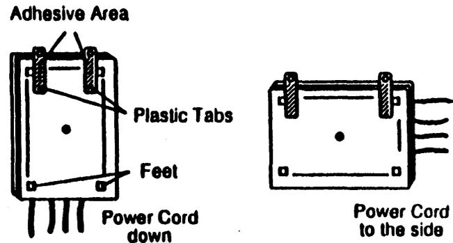
5. Press the tabs firmly into position.
