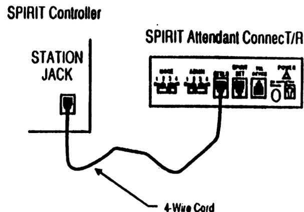
1. Connect the **SPiRiT** Attendant Connect/R to the Controller. Using 4-wire cord, plug one end into the CTRLR jack on the back of the **SPiRiT** Attendant Connect/R and connect the other end into the STATION jack on the controller.
