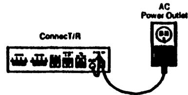
of the **SPiRiT** Attendant Connect/R. To prevent the power cord from pulling out easily, make a small loop of cord near the power connector and slip it behind the strain relief tab next to the POWER jack on the **SPiRiT** Attendant Connect/R. Plug the wall transformer into an AC power outlet that is at least 3 feet away from the controller and not controlled by a wall switch. (If it is any closer to the controller, you may hear a hum on your **SPiRiT** System.)
