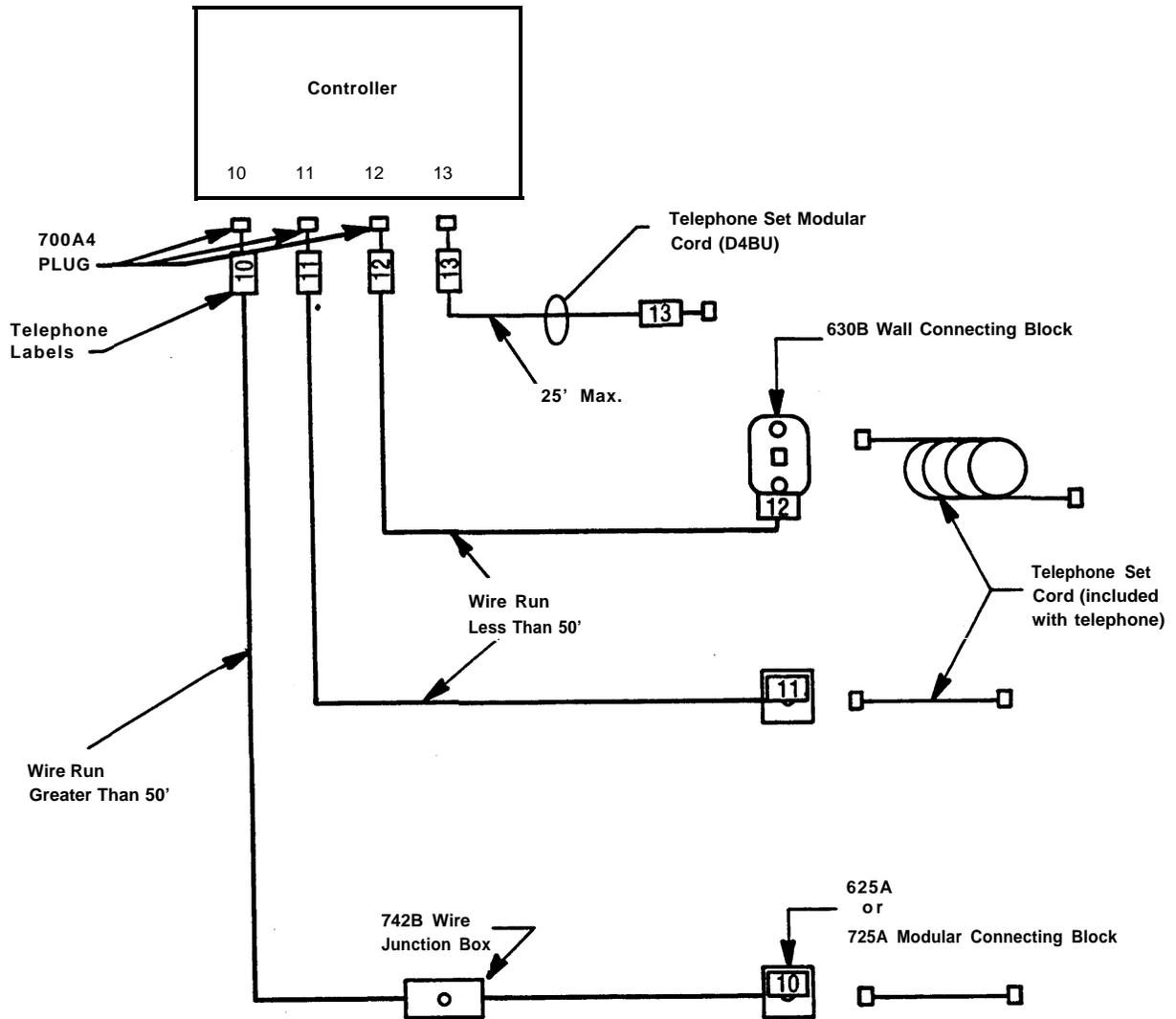
**Note to installers:** The SPIRIT system requires a reversal in the station set wiring. This reversal is in the telephone (tinsel) cord that is packed with the telephone, so all other station set wiring should be straight.
