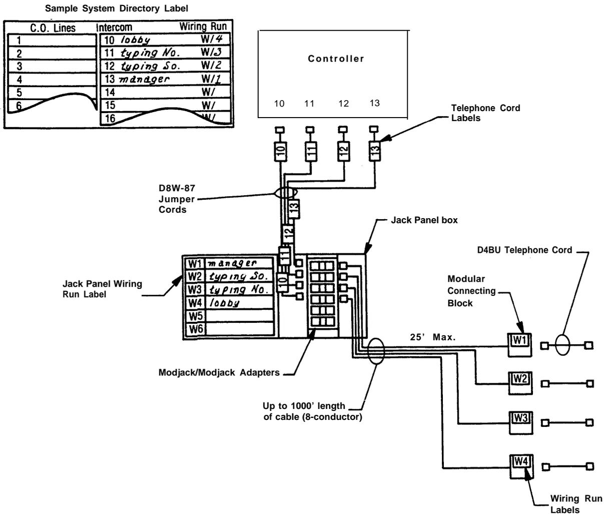
If you choose to wire your system with customer convenience wiring, use the wiring run labels to label *EACH END* of *EVERY* cord, as well as the wire junction boxes.
