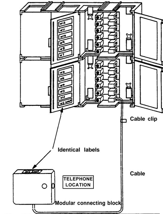
Finish your installation by routing cables to all other telephone locations and installing modular connecting blocks for each one. Be sure to label both ends of each cable run identically.
