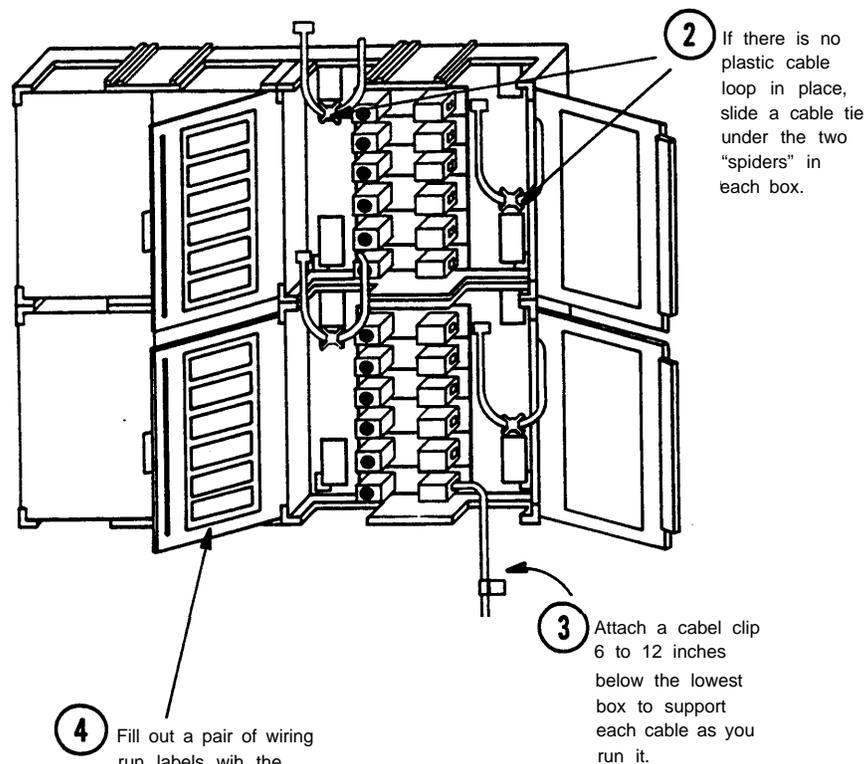
2 If there is no plastic cable loop in place, slide a cable tie under the two "spiders" in each box.
