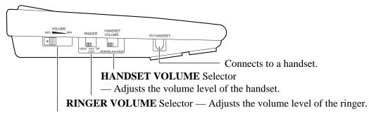
**VOLUME** Control — Adjusts the volume level of the speaker volume.
