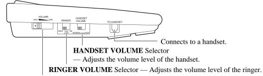
**VOLUME** Control — Adjusts the volume level of the speaker volume.
