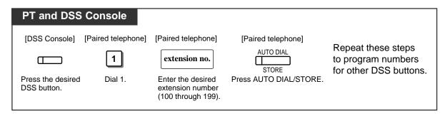
— To exit the Station Programming mode, set the MEMORY switch to "SET".
