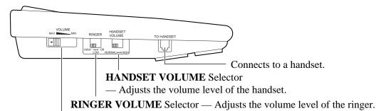
**VOLUME** Control — Adjusts the volume level of the speaker volume.
