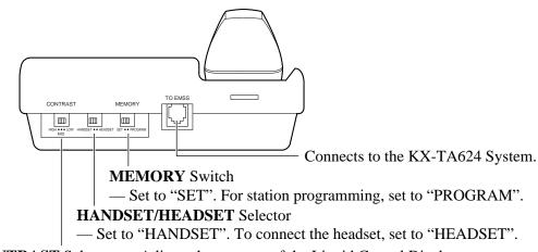
**CONTRAST** Selector — Adjusts the contrast of the Liquid Crystal Display.
