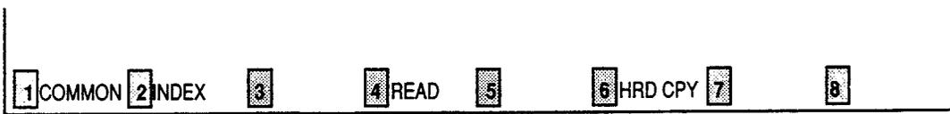
COMMON (SHOW LV, CHG LV, INS, OUS, REMOVE, EXIT) and HRD CPY keys are available in all setting screens. INDEX and READ keys are also available in this screen. The operation of function keys are described in Section 7-1 "Operation of Function Keys." Only messages are provided here.
