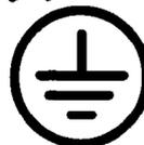
3. This grounding conductor is referred to as the telecommunications ground or supplementary ground as permitted in Section 250-91 (c) of the NEC. This shall be an insulated #6 AWG, green or green and yellow striped wire which is to be connected to the grounding stud within the cabinet. The following symbol is located adjacent to the stud to identify the connection point for the system grounding conductor:
