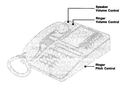
Before using your SUPERSET 4, you may want to adjust the Speaker Volume and Ringer Volume Controls and the Ringer Pitch Control. By adjusting the Ringer Pitch Control, you can identify more easily whose phone is ringing because the phones will ring at different pitches.
