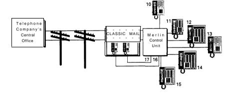
Because the CLASSIC MAIL system has been designed to plug into unused voice terminal jacks, the electronic circuits in the CLASSIC MAIL system are recognized by the Control Unit as additional Merlin telephones. Figure 1B shows the CLASSIC MAIL system unit plugged into voice terminaljacks 16 and 17 of a Merlin Control Unit. The CLASSIC MAIL system's unique ability to emulate a Merlin telephone is referred to as a *telephone emulation*\*.
