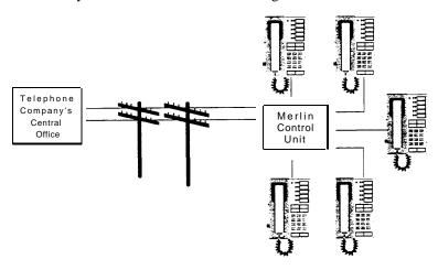
Figure 1A. Typical Merlin System
