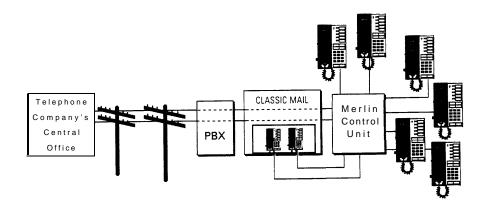
Figure 4H: Installing the CLASSIC MAIL system behind a PBX telephone system
