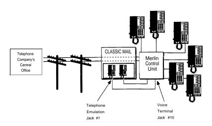
Figure 4G: Installing the CLASSIC MAIL system when using "Message" lights
