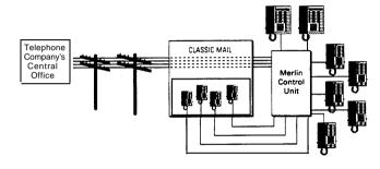
Figure 4A: Typical Expanded CLASSIC MAIL System Installation
