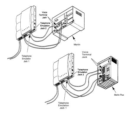
Figure 3F: Connecting telephone emulation lines to the Merlin Control Unit
