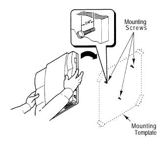
Figure 3A: Properly located mounting fasteners, with the CLASSIC MAIL system being positioned
