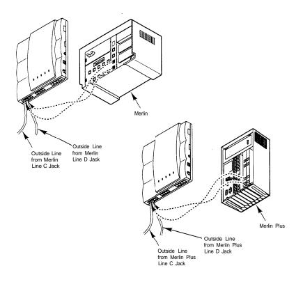
Figure 3B: Reconnecting outside lines from Merlin
