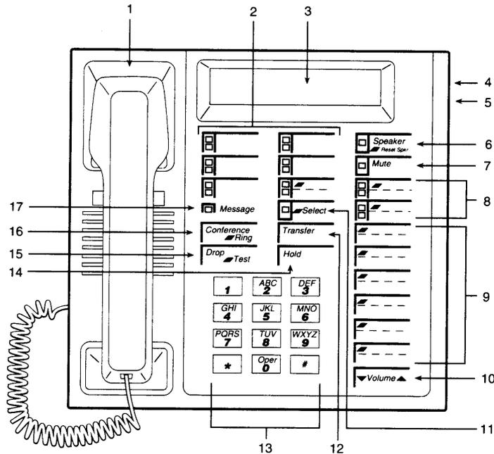
**Figure 1. 7406 Plus Voice Terminal (With Display)**
