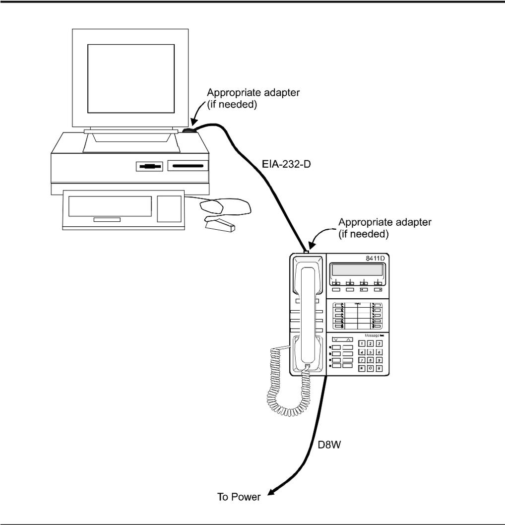
**Figure 1-4. Connecting the PC to the 8411 Telephone**
