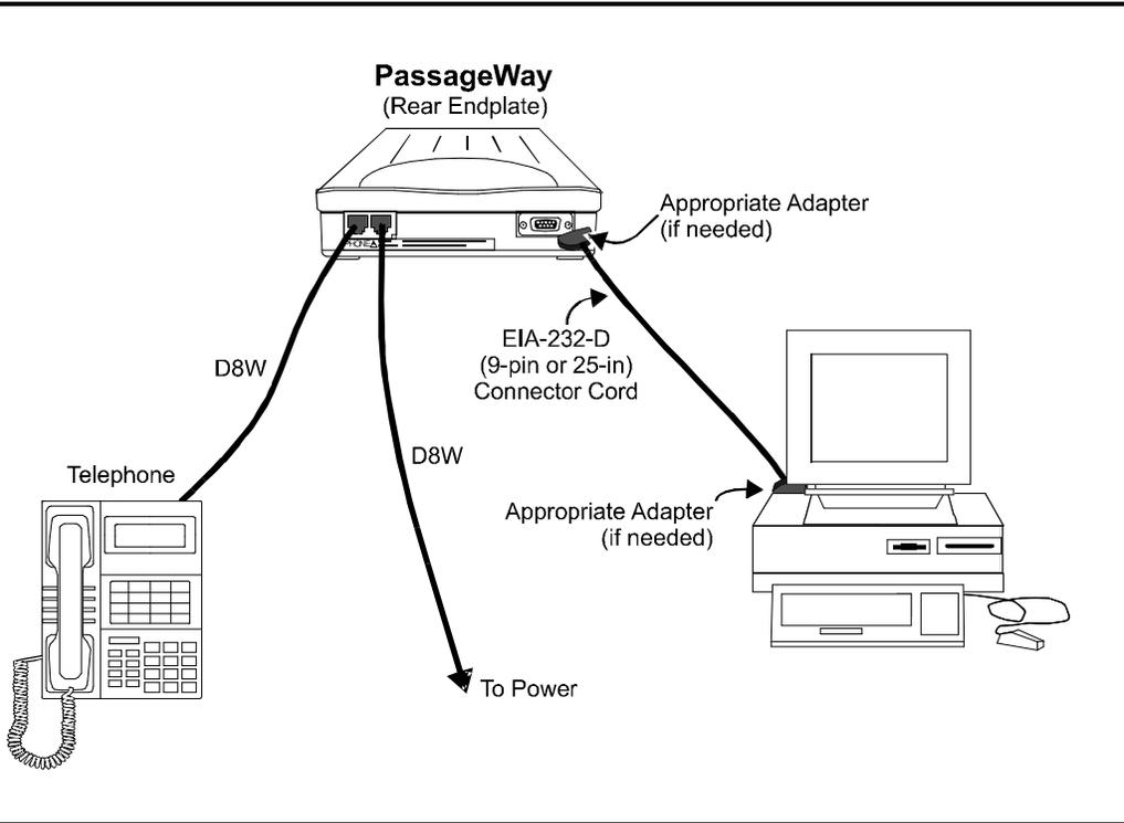
**Figure 1-5. Connecting the PC to the DCP Telephone and PassageWay Adapter**
