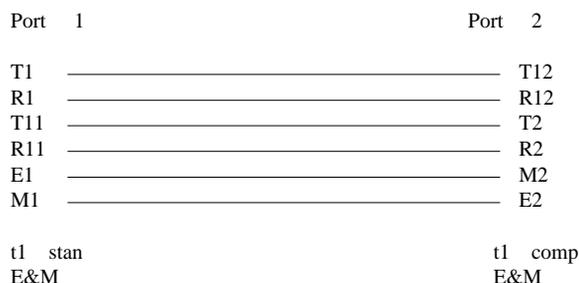
13. Check all wiring to verify good connections between the two test ports.
