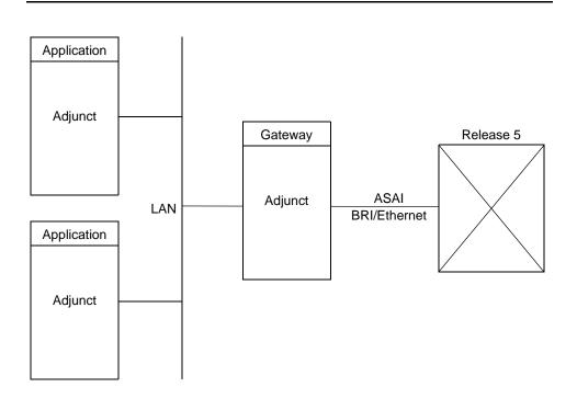
Figure 2-4. Single Link — Gateway/Server Configuration
