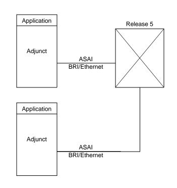
Figure 2-3. Single Link — Multiple Processors Configuration
