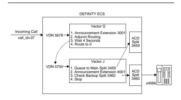
Figure A-15. Call Flow for Call to a VDN with Announcement and Routed to Another VDN
