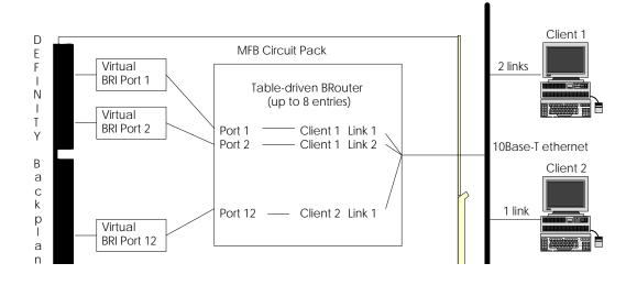
Figure 13-4. Relationship of Virtual BRI Ports, Brouter, and DEFINITY LAN Gateway Clients
