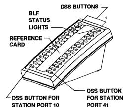
When a DSS/BLF console is initially connected at a station port, the system recognizes it as such, and automatically assigns the station intercom numbers to the console buttons for the maximum number of stations connected to the system. (The maximum coverage is limited by the 32 available buttons.)
