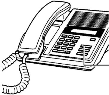
The memory button can store a telephone number or feature code to give you one touch dialling or feature activation. You can change the memory button by programming it with a new number or feature code.
